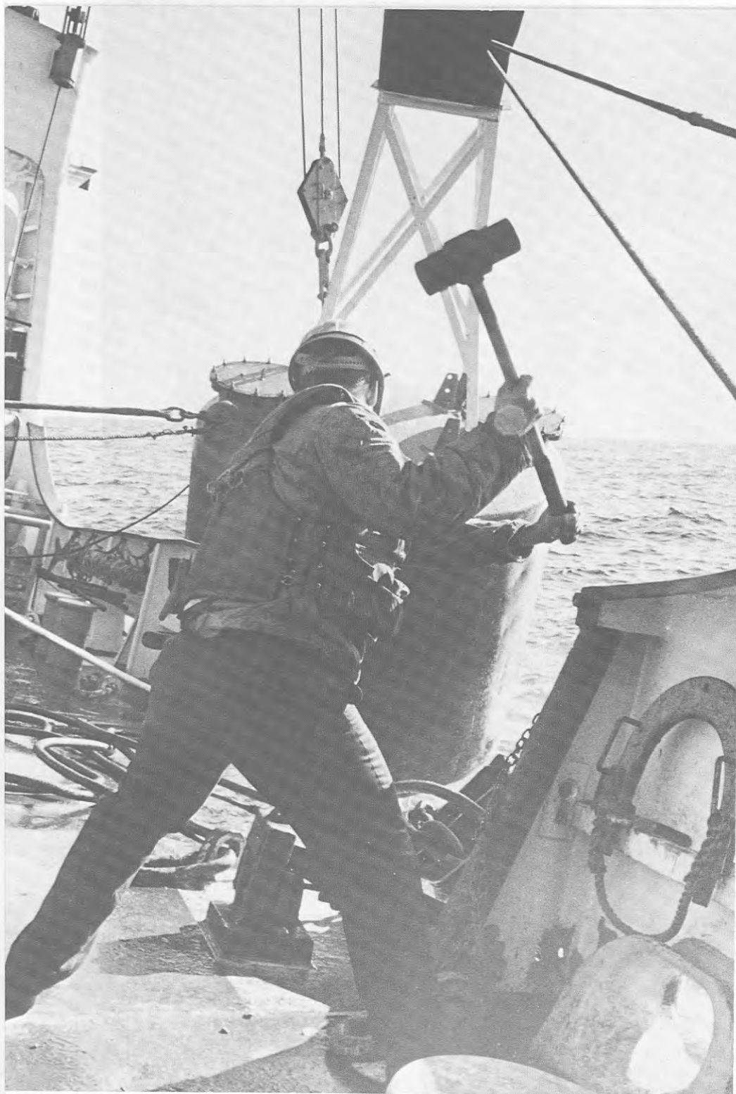
Buoy tender crewman stands ready to trip the chain stopper.
