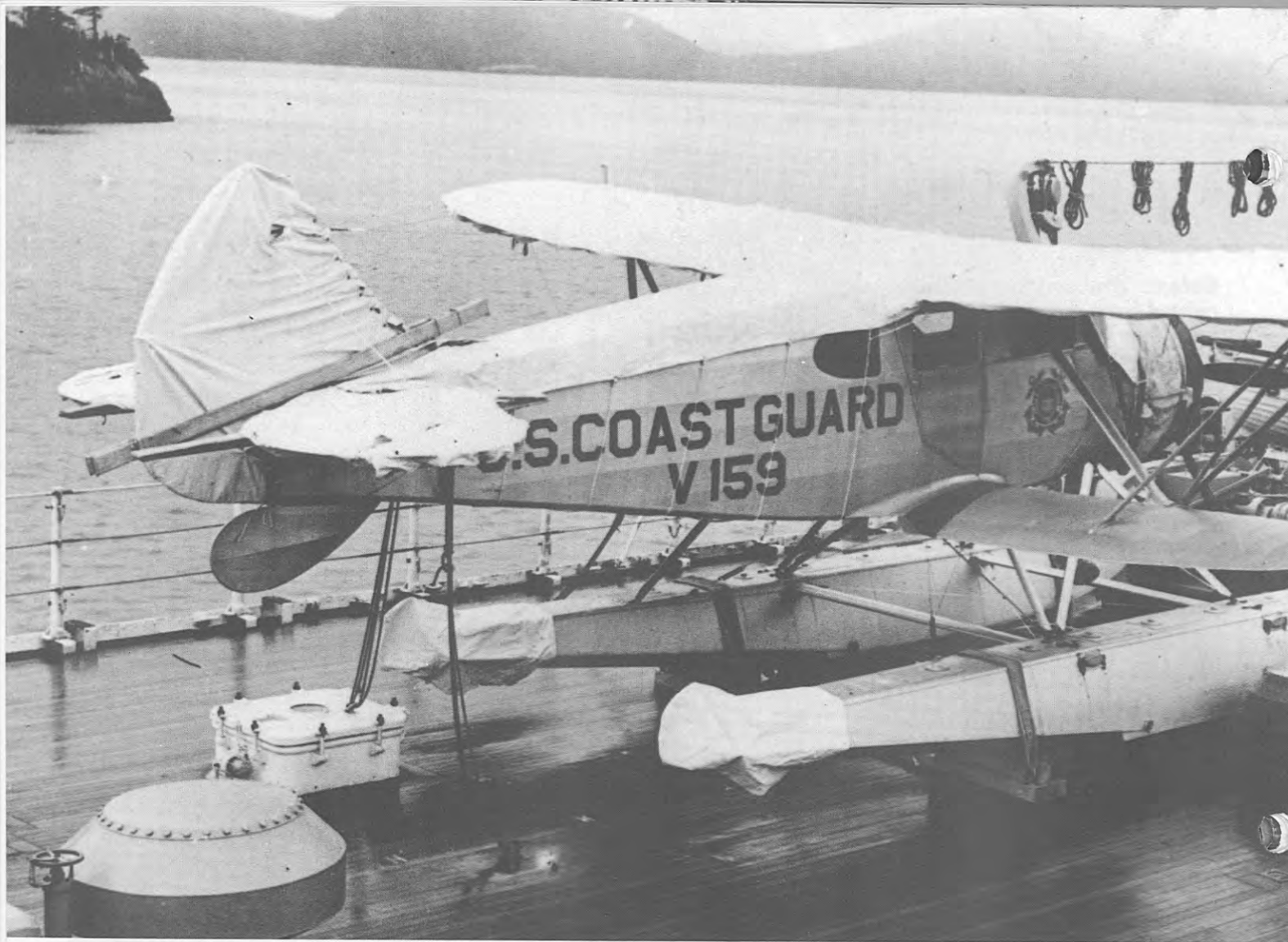
A J2W-1, secured for sea, is shown here on board the Spencer at Cordova, Alaska, in February 1938. These aircraft were used with floats or wheels or fitted with skis for takeoffs and landings on ice.
