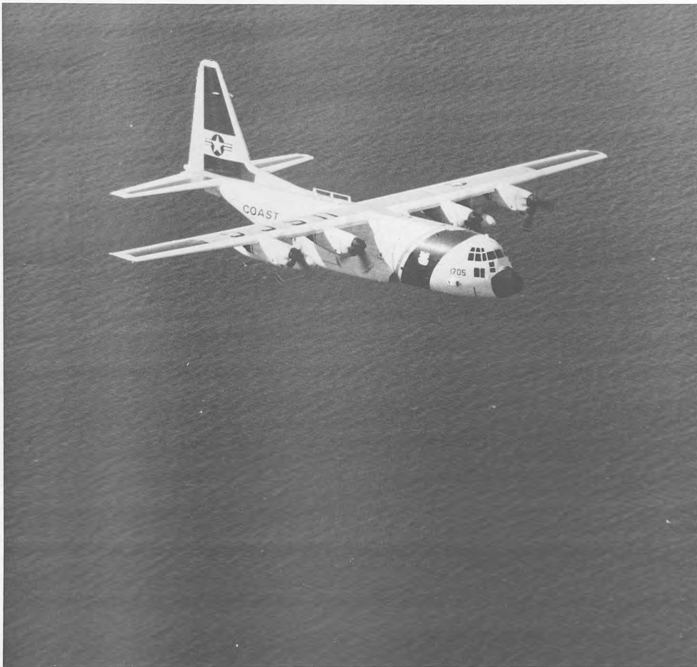
The HC-130H, a long range surveillance and transport aircraft, is the newest series of HC-130 model aircraft in use. Coast Guard crews have flown the Hercules since 1959.
