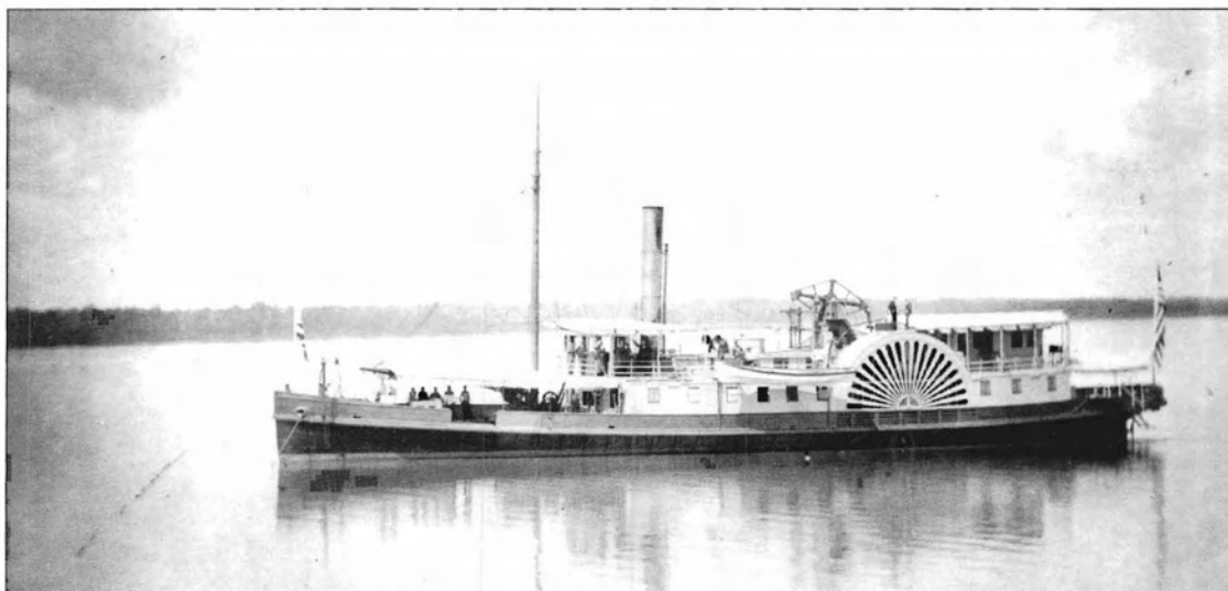
The USLHS Jessamine as it appeared in 1885. A side-wheel steamer with a walking beam engine, the Jessamine served primarily as a supply vessel for lighthouses. It was not, however, above doing the tough job of tending buoys.
