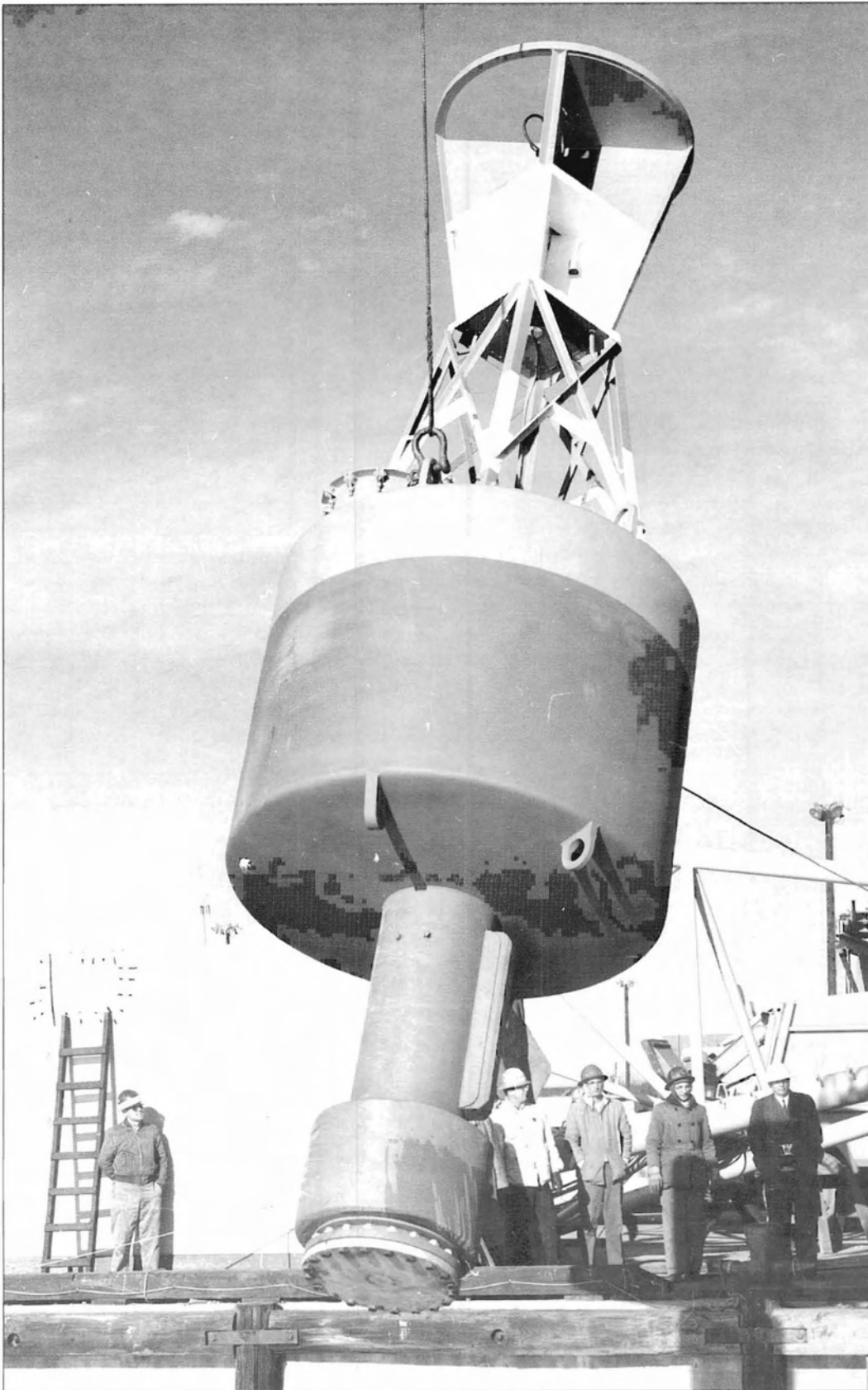
The Atomic Buoy was tested in Baltimore Harbor in 1961. It came complete with a SNAP-7A Strontium 90 generator. The buoy received world-wide attention and was presented as a model for the peaceful use of nuclear power. The generator, however, failed to keep the buoy lit. It was never deployed to its permanent station.
