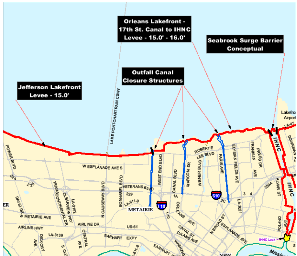
This is a detail of the recently-released 100-Year Design Elevation Map. It shows the heights that levees and floodwalls in the Hurricane and Storm Damage Risk Reduction System will be in 2011. The new map is available on the Corps' Web site at: http://www.mvn.usace.army.mil/hps/100yr_design_map.html
