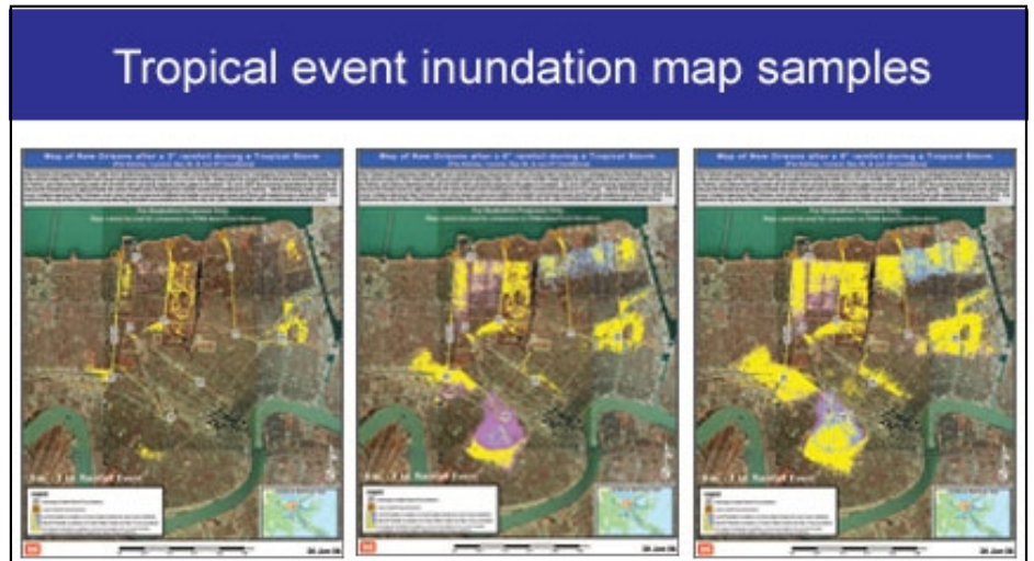
The inundation maps compare possible rainfall events and accumulations of interior water if the area were to experience 3-, 6- and 9-inches of rainfall over a six-hour period with the interim outfall canal gates closed. The maps are intended for illustrative purposes only. These maps cannot be used for comparison to FEMA Base Flood Elevations. For detailed information on the inundation maps, go to www.mvn.usace.army.mil/inundation_maps.htm
