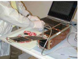
(U) Weather Colony Program CubeSats undergoing Payload Accommodation Study at the Naval Research Laboratory to determine candidate configurations for placing space weather sensors on a CubeSat.
