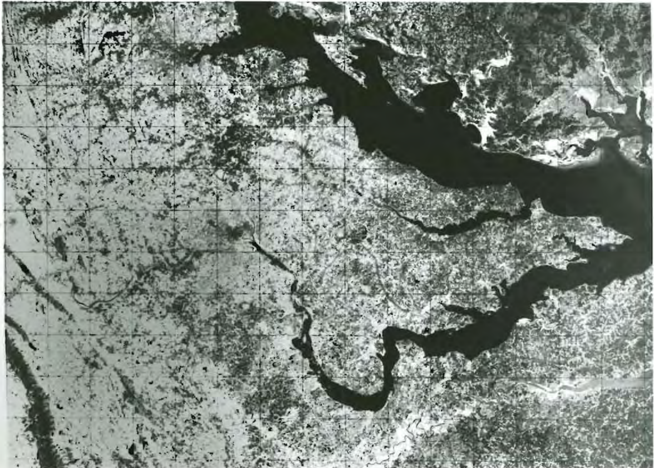
Fig. 1-27 — KH-4 Mapping Camera System imagery from stellar/index (S/I) camera (CORONA-MURAL); contact and 5x enlargement
