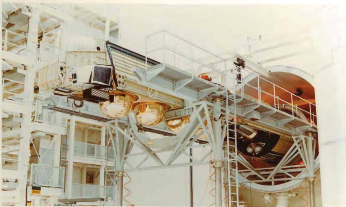
Fig. 2-28 — SV entering vacuum chamber
