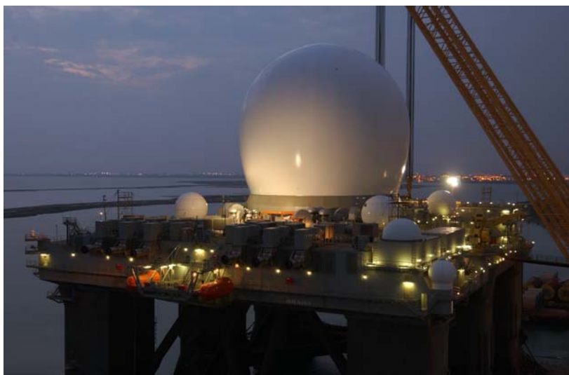
The Sea-Based X-Band Radar prepares to depart for testing in the Gulf of Mexico.
