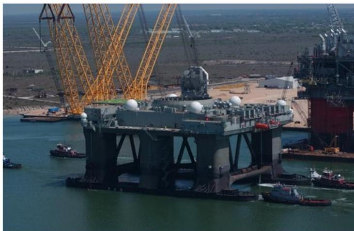
The Sea-Based X-Band Radar platform arrives at Kiewit Offshore Services in Corpus Christi, Texas on March 17, 2005. While at Kiewit, the 2,000 ton X-Band Radar (seen directly behind the platform) will be lifted onto the platform later this spring.
