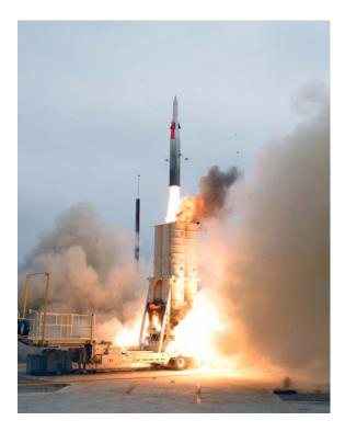
An Arrow anti-ballistic missile is launched as part of the ongoing United States/Israel Arrow System Improvement Program. The missile intercepted a short-range target west of San Nicolas Island on the Pt. Mugu Sea Range in California. This was the twelfth Arrow intercept test and the seventh test of the complete Arrow system (US Navy photo).
