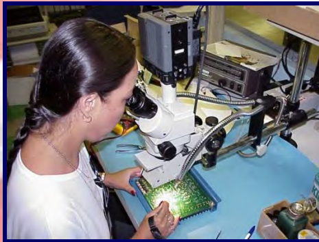
Multi-Layer Circuit Card Testing and Repair
