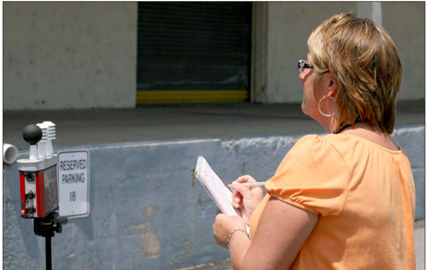
Annette Feie takes a reading of the Wet Bulb Globe Temperature Heat/Stress Monitor after it has calculated the temperature. Two meters are set up to ensure a more accurate reading.
