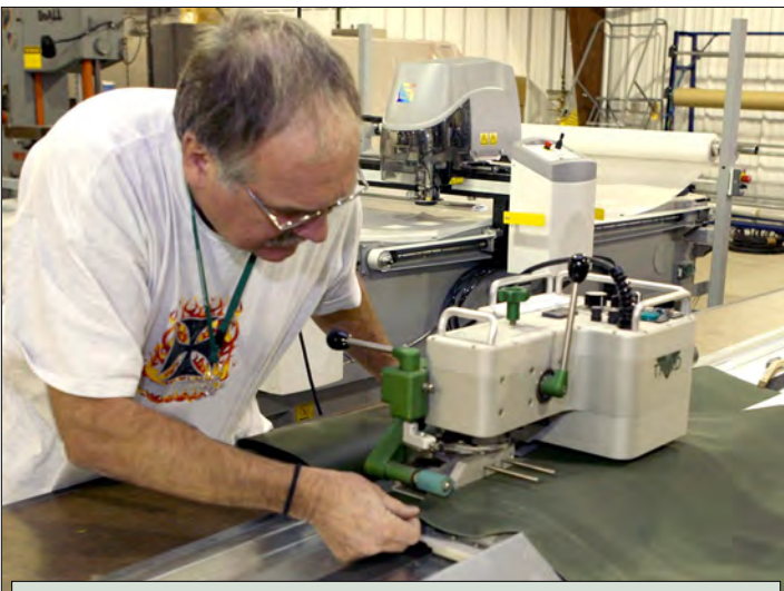
Gregory Funk utilizes the Vinyl Welder for making covers of Containerized Kitchens (CK).
