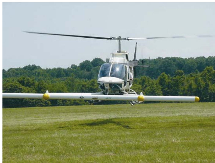
Figure 3c. MTADS Kit on Helicopter
