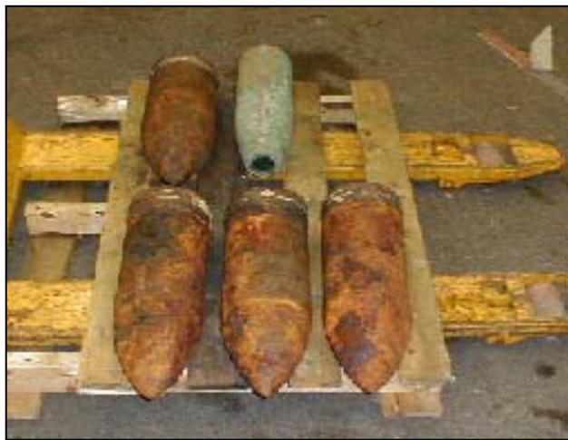
Photos 1 & 2: WW-I and WW-II era coastal defense 6-inch projectile underwater south of Oahu, Hawaii ( top ) and recovered shells from the same area with encrusting growth removed ( bottom ).
