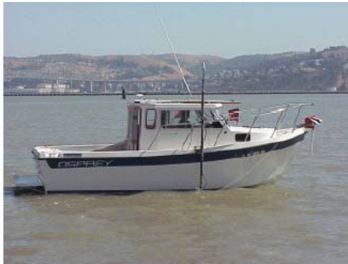
Photo 9. Seafloor Systems' deployed sonar system..
