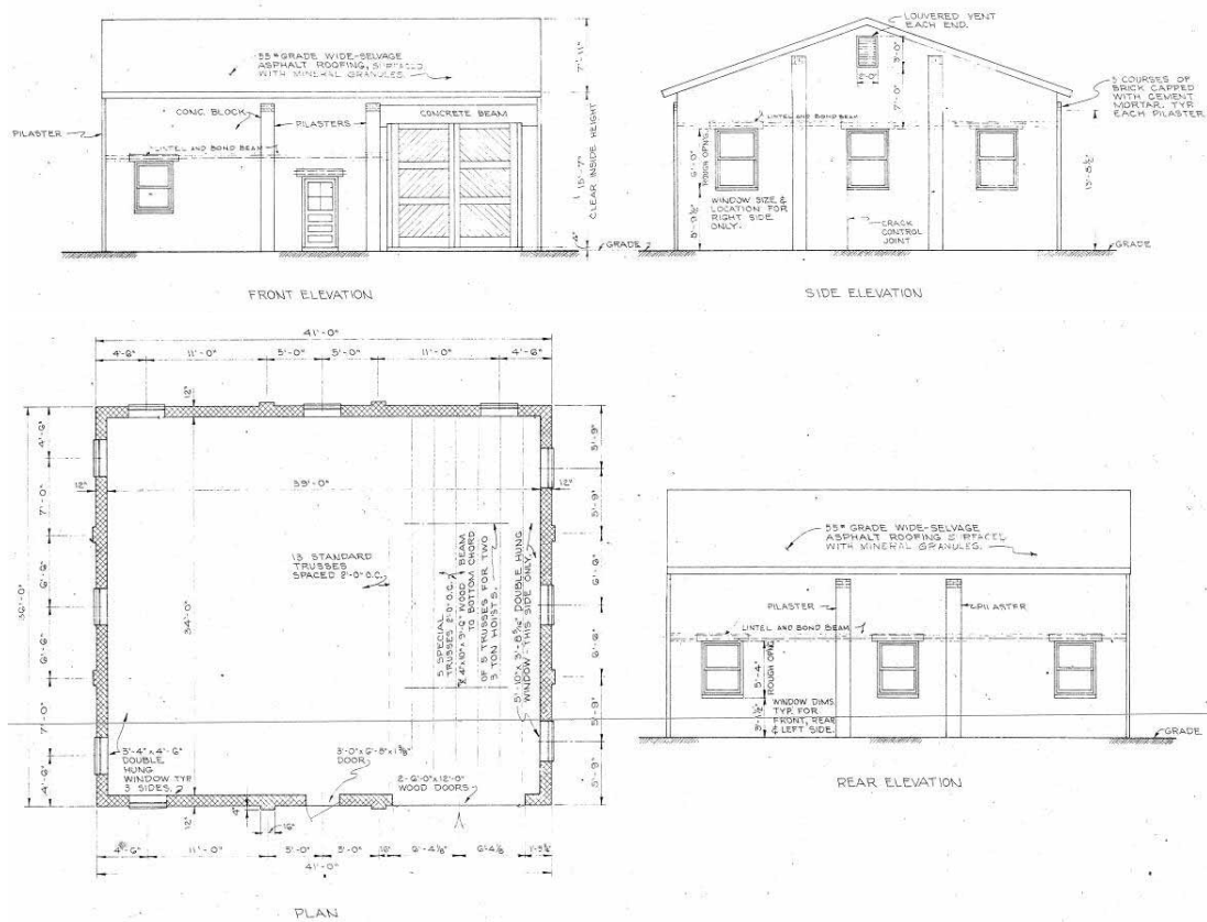
Figure 68. Floating bridge area, masonry covered storage building, plan and rear elevation, Fort Bragg, NC, 1952 (Standard Drawing 28-13-97 Sheet 2 of 4, "Bridging area, floating bridge, covered storage building-masonry," 19 May 1952).
