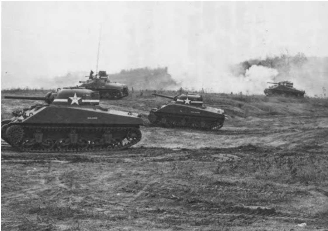
Figure 202. M-4 tanks each with a 75 mm gun at Fort Knox, KY, December 1942 (NARA College Park, RG 111-SC WWII, box 107, photo SC150392).
