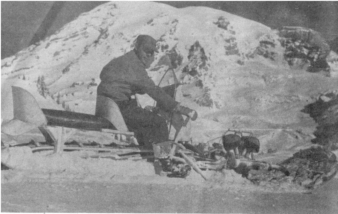
THE ELIASON MOTOR TOBOGGAN TESTED ON MT. RAINIER. THOUGH SPEEDY ON PACKED SNOW, THIS MACHINE PROVED UNSATISFACTORY IN HEAVY POWDER. IT WAS LATER REPLACED BY THE M-28 AND THE M-29.
