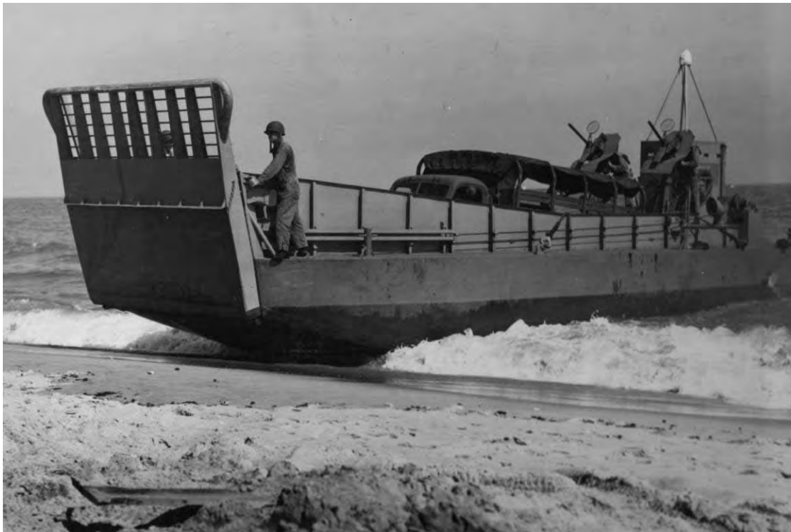
Figure 222. A landing craft, mechanized (LCM) with a load of one truck in training operations on the Atlantic coast with Mark 21-30 caliber machine guns, 21 August 1943 (NARA College Park, RG 80-G, box 393, photo 85158).
