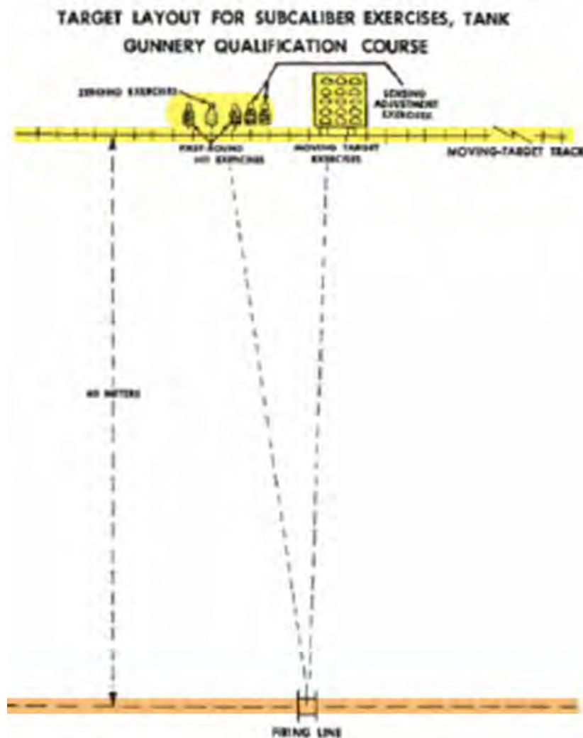
Figure 218. Single subcaliber range layout, circa 1961 (FM 17-12, Tank gunnery, 3 April 1961, pp 339, 342).
