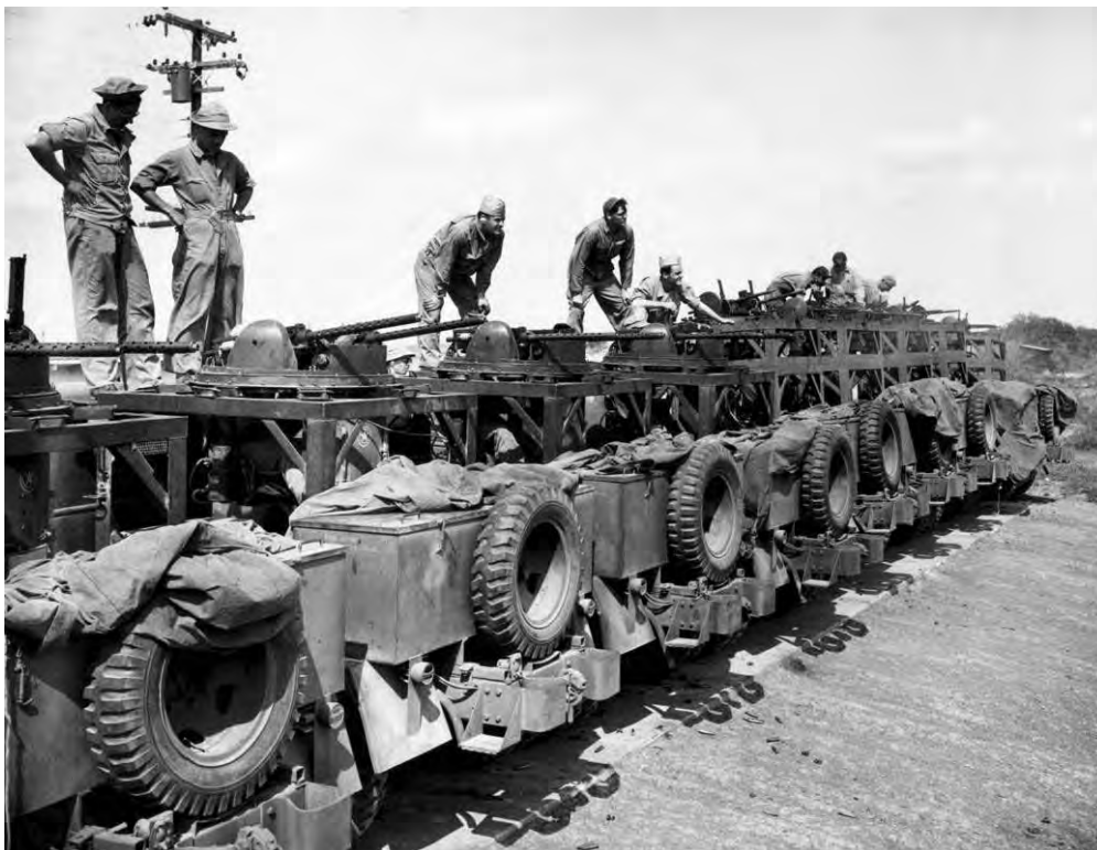
Figure 22. From turrets mounted on trucks, aerial gunnery students fire at stationary and moving targets at Harlingen Army Air Field, TX, June 1943 (NARA College Park, RG 342-FH, box 2202, photo 4A-17282).
