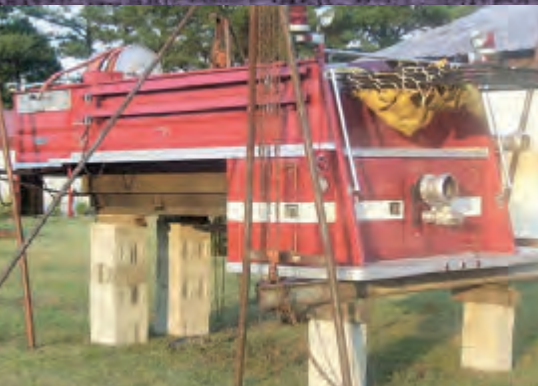
Members of North Carolina's South Edgecombe Rural Fire Department built the above fire truck by combining an existing fire truck with a 5-ton Army truck the department received from DLA Disposition Services. Volunteers spent nearly 700 hours outfitting the truck with 125 hose and pipe fittings, 350 feet of wire, 75 light bulbs and nine gallons of paint. Images to the left show various stages of construction.
