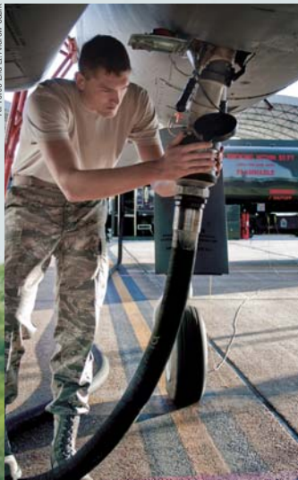
Air Force Senior Airman Jacob Prine checks the fuel connection to an F-15 prior to a flight test of new environmentally friendly fuel. DLA is helping lead the way in alternative fuel procurement throughout the services.
