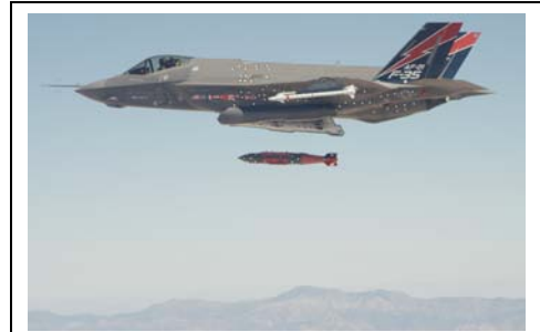
An F-35A conventional takeoff and landing (CTOL) aircraft completed the first in-flight weapons release of a 2,000 pound GBU-31 BLU-109 Joint Direct Attack Munition (JDAM) from a 5th Generation fighter, Oct. 16. (Photo courtesy of Lockheed Martin)
