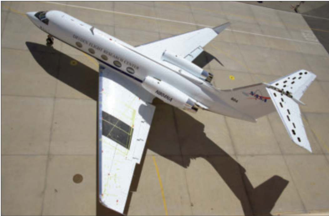
A NASA experiment will be flown on this jet to test improving laminar flow over an aircraft wing. The marked area on the left wing shows the area where an experimental glove will be located. Image credit: NASA/Tony Landis.
