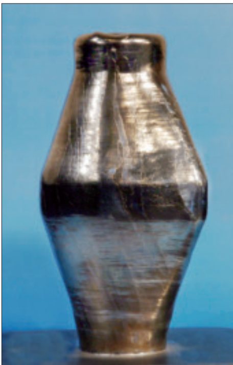
The electron beam free form fabrication process was used to make this sample titanium part. NASA innovators are working on scaling up the process to build larger components. Image credit: NASA.
