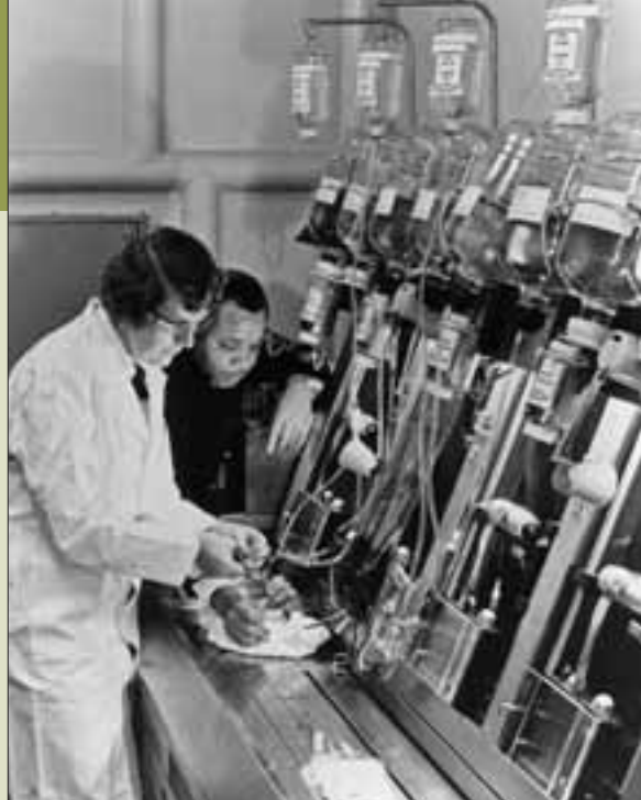
Lieutenant Commander Edna McCormick and Hospital Corpsman Chief H. E. Williams use a cytoglomerator to reconstitute frozen blood aboard Repose (AH 16).
