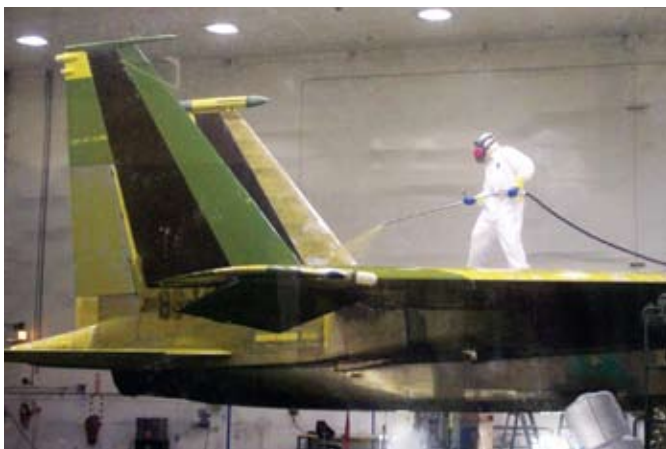
Manual Alodine application uses over 100 fewer gallons than an automated gantry system.
