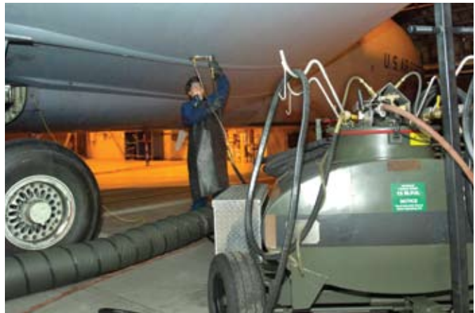
A "Sealvac" unit is installed to drastically reduce fuel spills on aircraft during inspection and repair.
