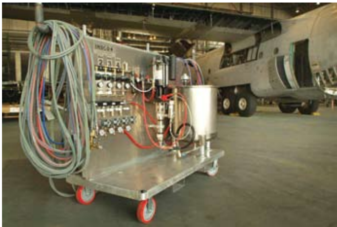
The Air Assisted Airless Spray Paint System resulted in a 40 percent reduction in paint primer and topcoat usage.
