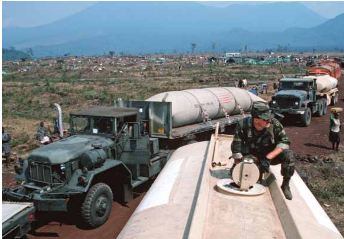
A member of a U.S. Army water purification team kneels on top of water truck, preparing to draw water from Lake Kivu, then chlorinate the water and transport it to the Kibumba refugee camp near Goma, Zaire, (now the Democratic Republic of Congo) in December 1994. (U.S. Air Force photo by Master Sergeant Rose Reynolds)
