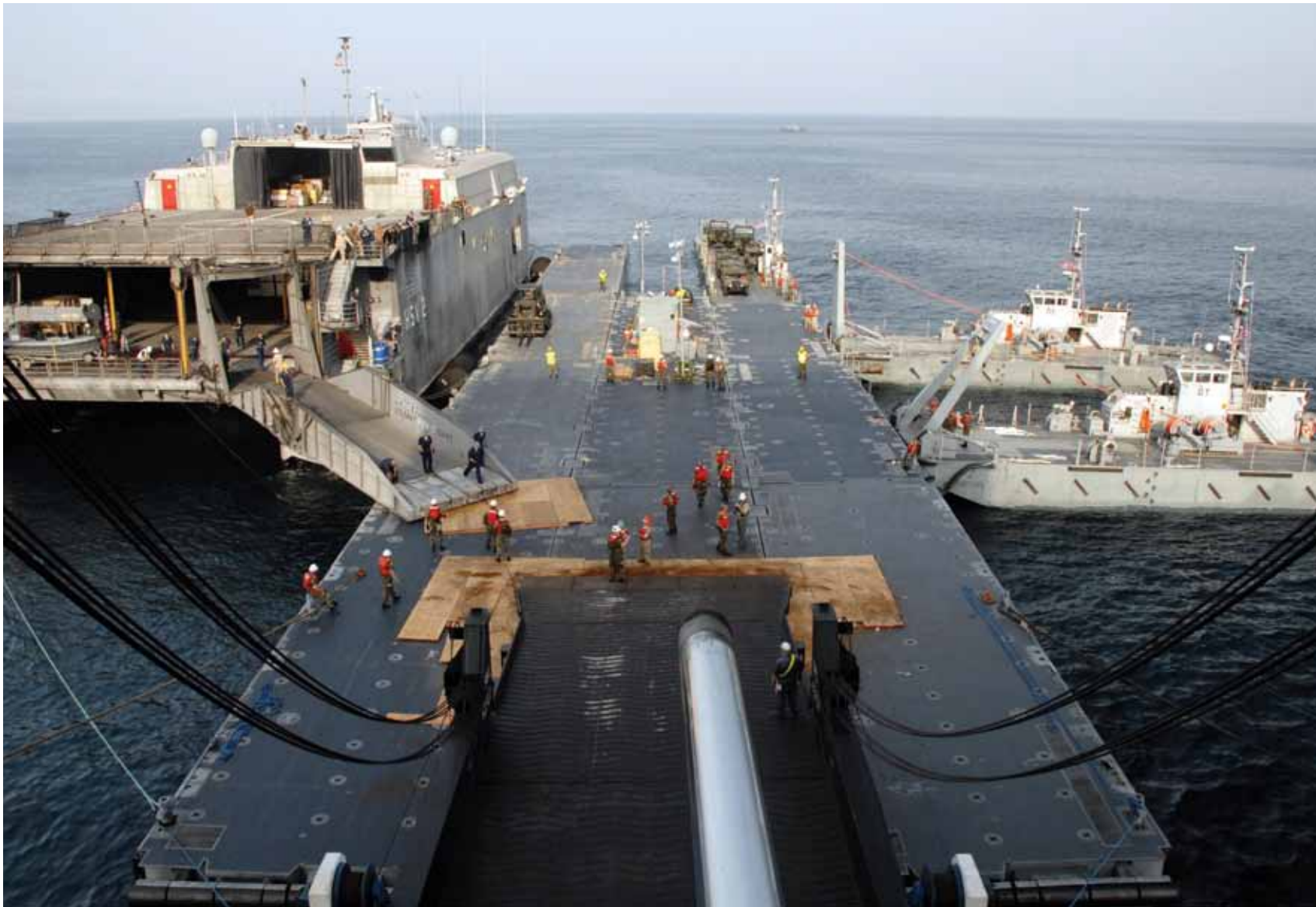
FLOATING DOCK - In the waters off Monrovia, Liberia, U.S. Navy and Marine Corps personnel construct the Improved Navy Lighterage System (INLS) during an exercise in March 2008. The INLS is a redesign of a floating dock system originally used during World War II. System pieces can lock together to create ferries, causeway piers, or roll-on, roll-off discharge facilities to transport cargo and equipment from ship to shore while leaving a minimal footprint, allowing the Navy to respond in areas without developed port facilities. (U.S. Navy photo by Petty Officer 2nd Class Elizabeth Merriam.)
