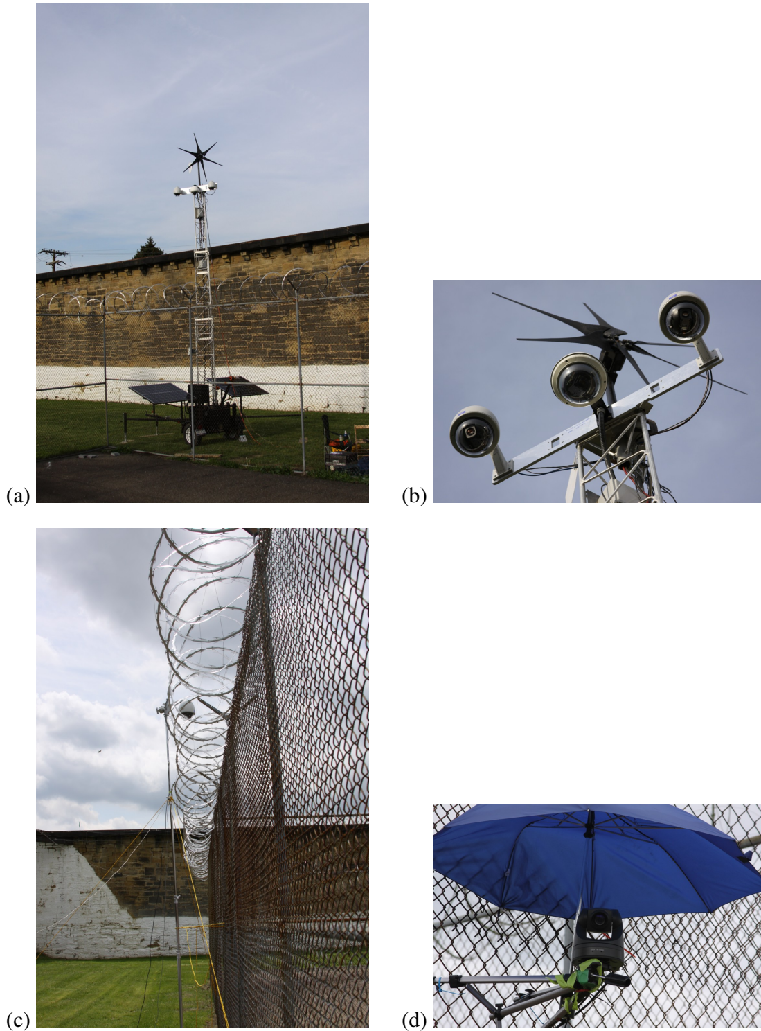
Figure 17: Cameras. (a) mobile tower with mounted cameras, (b) the left-most and right-most cameras belonged to the GE Global Research system, (c) broadcast tripod with mounted camera, and (d) computer controlled PTZ camera, mounted on fence.
