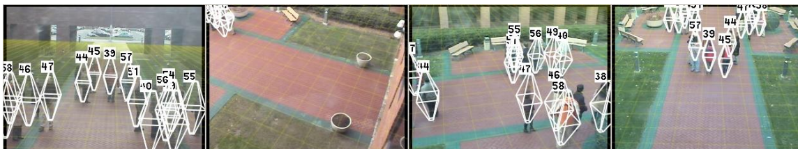
Figure 40: Large motion crowds: In this scene, there was a total of 23 individual subjects who were told to mingle in a 3-group configuration. The overlaid white wireframes with IDs show the tracking result from 4 fixed camera views.
