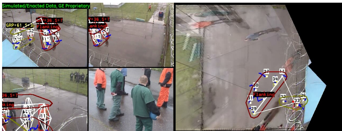
Figure 4: Flanking Detection. Example where the system correctly detected a FLANKING event and hence provided an alert to the operator before the subsequent fight ensued.
