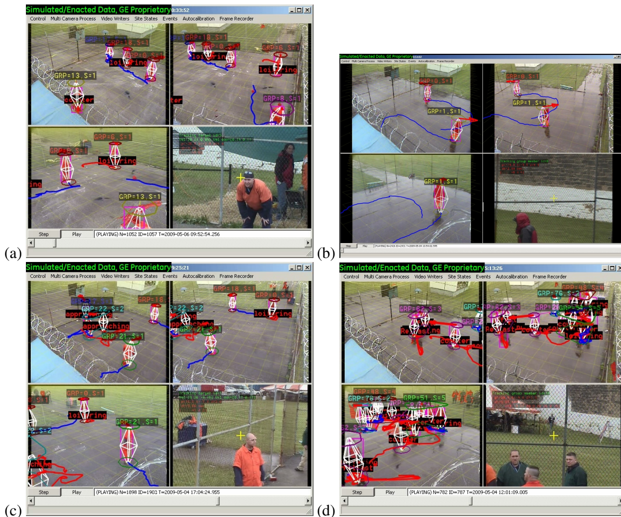
Figure 44: Tracking. The tracking system performed well even under crowded and active conditions: (a) actors playing dodge ball, (b) tracking in rain (notice the strong reflection of the person, which can sometimes lead to false person detections), (c) tracking during an actual scenario, and (d) tracking during a contraband exchange.
