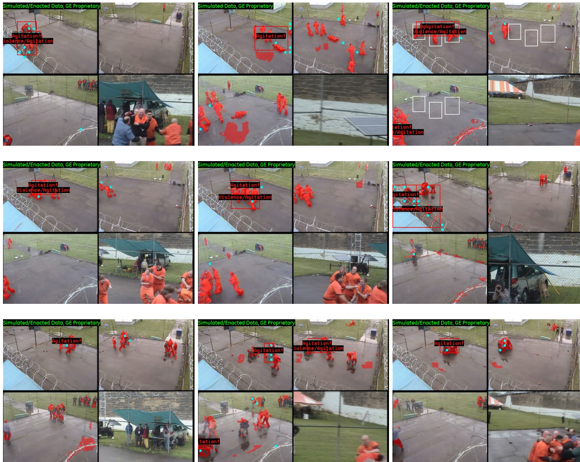
Figure 29: Aggression Detection. Nine example instances where the system detected a fight in progress. Every image contains red rectangles that outline the detected aggression region.
