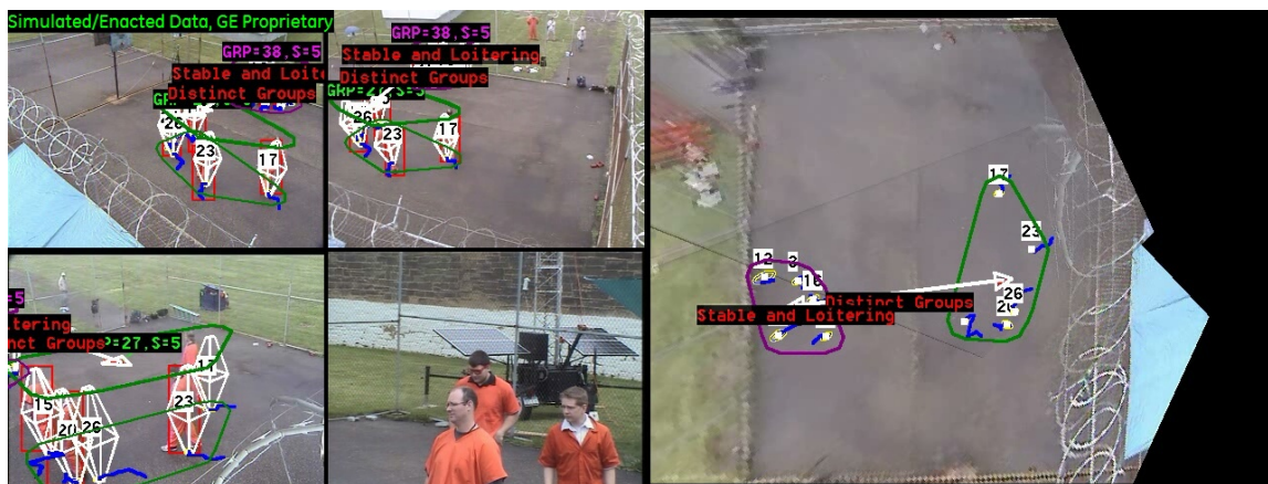
Figure 11: Distinct Group Detection. A detection algorithm has been developed that detects pairs of gangs that are stable and have certain spatial configurations with respect to one another. One group (red) is considered stable and loitering. It is considered to be distinct from the second group (green).
