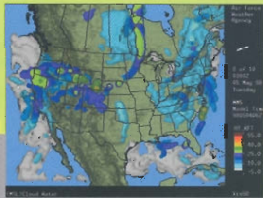
Two Dimensional Cloud Forecast from the MM5 (36 km resolution) CONUS Window, as visualized by Vis5D.
