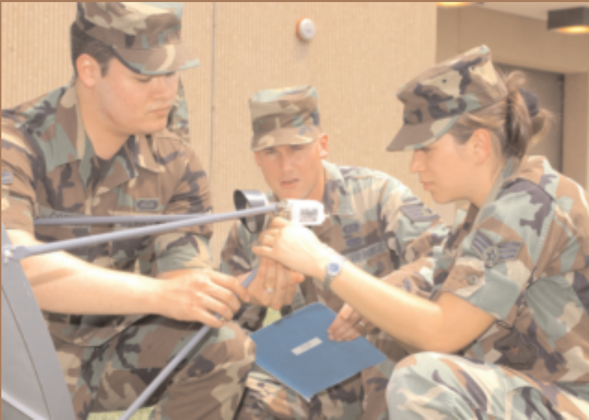
Airman 1st Class Jack Cotham (left), Staff Sgt. Charles Andrews and Senior Airman Micki Erdelac, combat weather students in the 335th TRS, assemble a tactical very small aperture terminal. The TVSAT transmits and receives large volumes of weather data via satellite. Photo by Ms. Kemberly Groue.
