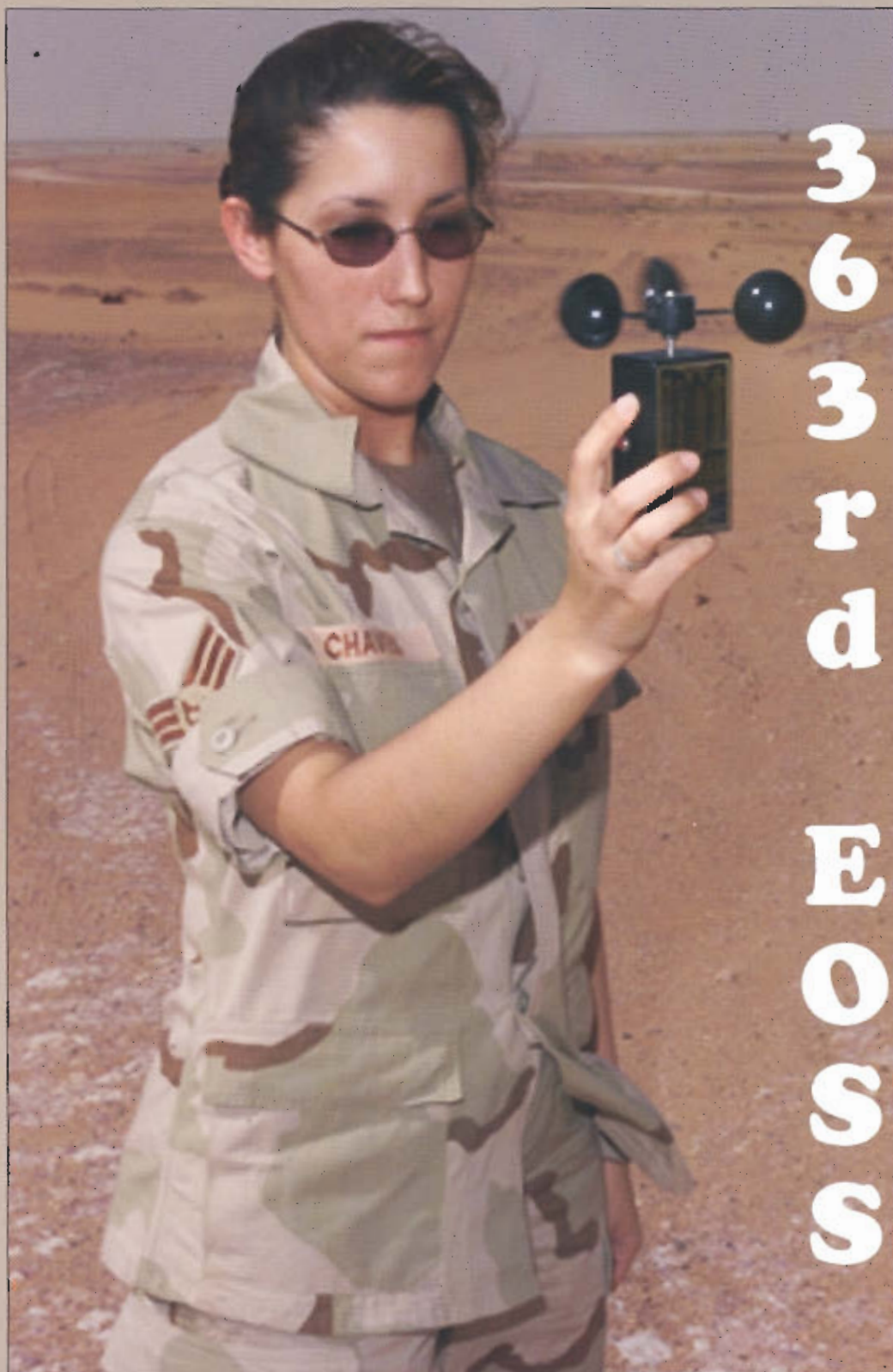
Senior Airman Debra Chaves, 363rd EOSS weather technician, verifies current wind speed using an anemometer. Chaves is currently deployed to PSAB from the 47th OSS/OSW, Laughlin AFB, Texas, in support of OSW.
