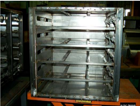
600 CFM Gas Filter Assembly Housing (with filter trays removed)
