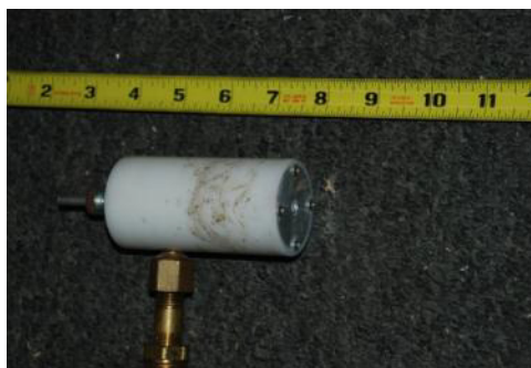
Figure 1. SRI-nozzle used to disseminate the test powders.
