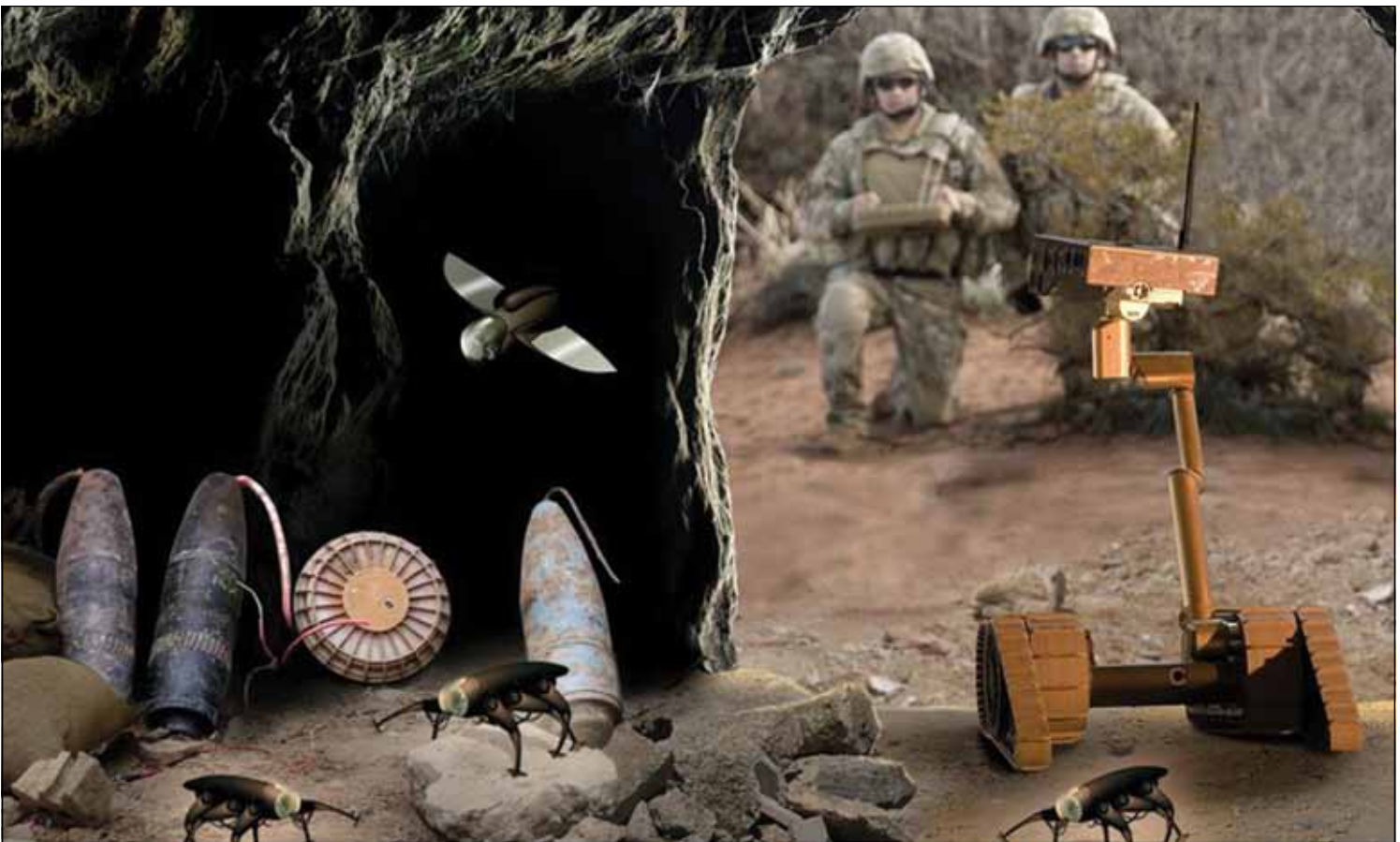
Air and ground MAST systems work with a relatively larger Small Unmanned Ground Vehicle. (Illustration courtesy of ARL.)
