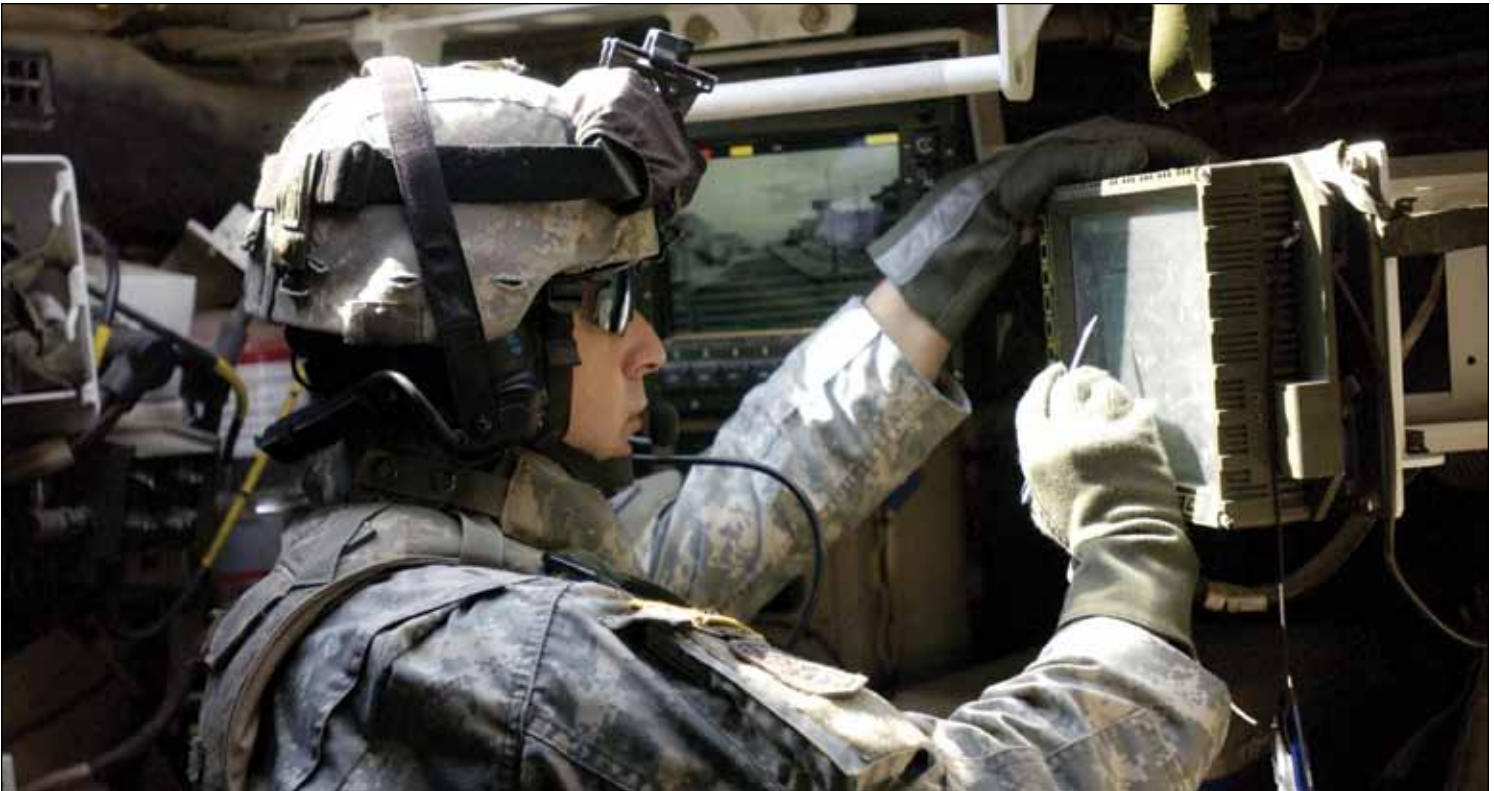
A Soldier uses Force XXI Battle Command Brigade and Below to plot the position of friendly forces. (U.S. Army photo courtesy of PEO C3T.)
