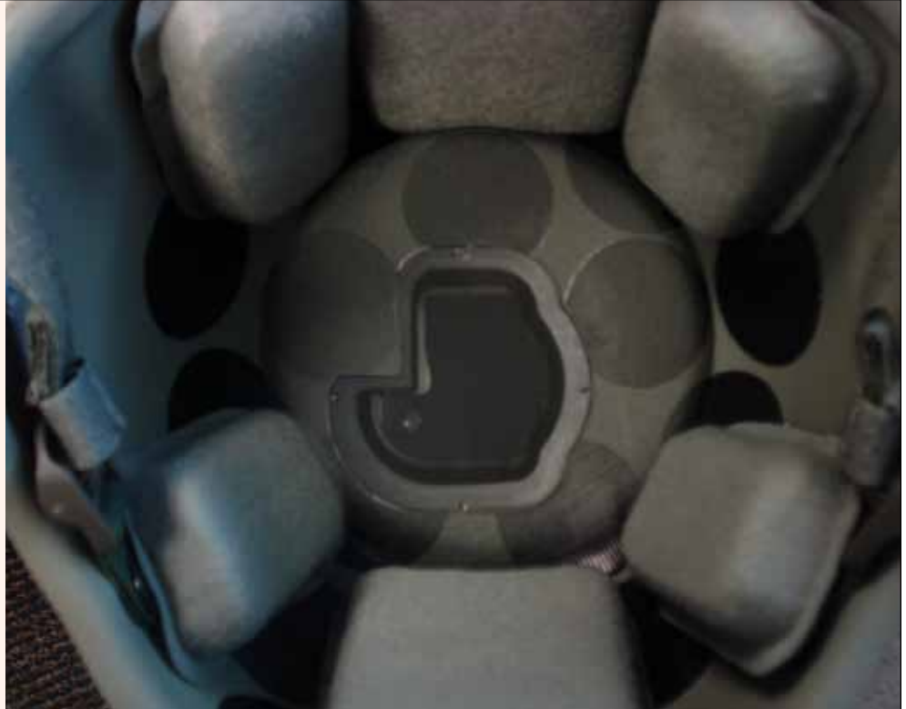
The Helmet Sensor Program provides small, lightweight, low-power sensors that mount to Soldiers' combat helmets. The sensors detect, measure, and record impact and blast overpressure associated with IEDs and other events that may cause concussions in an operational environment. (U.S. Army photo courtesy of PEO Soldier.)
