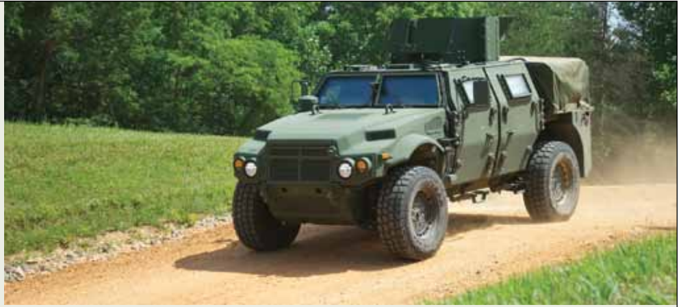
Testing is an area where potential economic efficiencies can be gained. Here, the Joint Light Tactical Vehicle undergoes a dirt track test at the Churchville Test Area near Aberdeen Proving Ground, MD, June 3, 2010. (U.S. Army photo by David McNally, U.S. Army Research, Development, and Engineering Command Public Affairs.)
