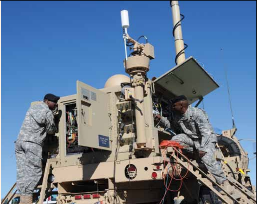
CW5 Leslie Cornwall (left) and MAJ Marcus Odom from the U.S. Army Training and Doctrine Command Capabilities Manager Networks and Services examine Warfighter Information Network-Tactical (WIN-T) equipment during the WIN-T Increment 2 Engineering Field Test at Fort Huachuca, AZ, in December 2008. (U.S. Army photo by Richard Mattox, Program Executive Office Command, Control, and Communications-Tactical.)
