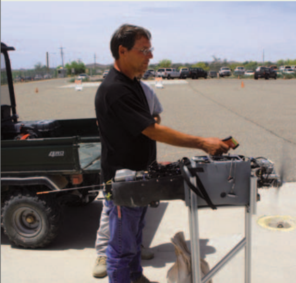
YPG Test Officer Bill Loftis measures the temperature of an unmanned aircraft’s motor. (U.S. Army photo by Mark Schauer.)
