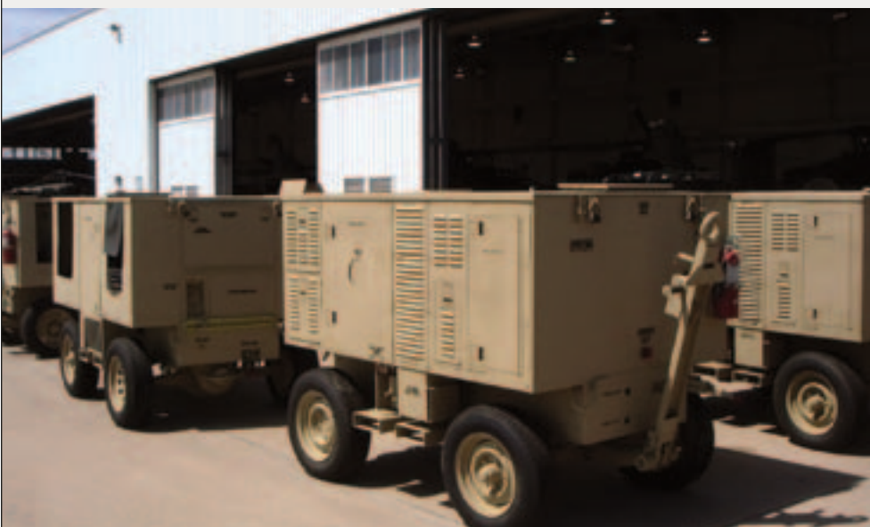
The Aviation Ground Power Unit provides AC/DC electrical, hydraulic, and pneumatic service for all Army rotary-wing aircraft. (Photo courtesy of PM AGSE.)
