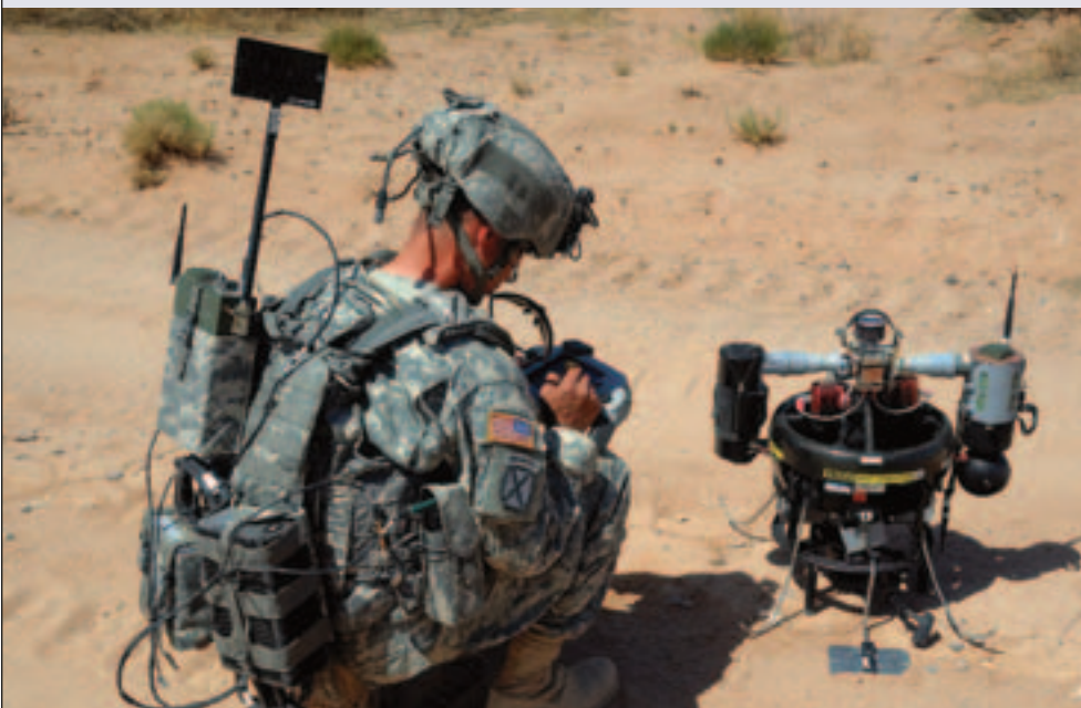
A Soldier equipped with a Common Controller conducts a pre-launch check of a Class 1 Unmanned Aerial Vehicle (UAV). The Common Controller consolidates control of numerous sensor nodes and unmanned systems, including the Class 1 UAV and the Small Unmanned Ground Vehicle, into a single integrated networked controller. (U.S. Army photo.)
