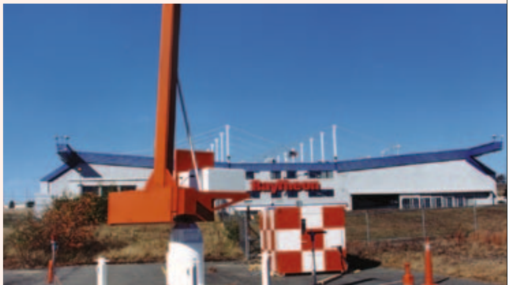
The AN/FPN-67 Fixed-Base Precision Approach Radar serves as the U.S. Army’s primary aid to recover aircraft to fixed-base airfields during adverse weather. (Photo courtesy of PM ATC.)
