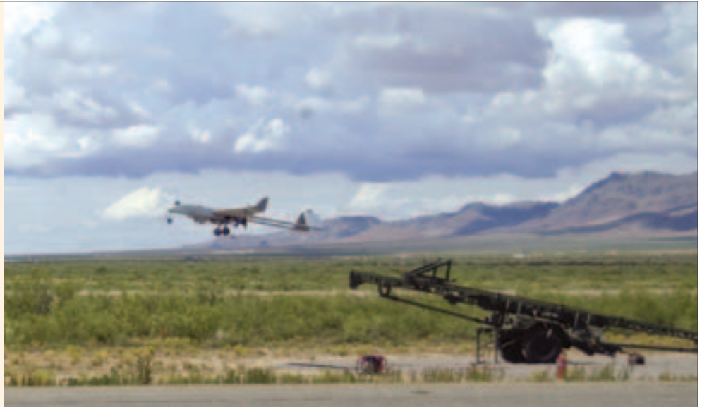
A Shadow unmanned aerial vehicle is launched from Condron Field, WSMR, NM. The Shadow is equipped with various camera systems to provide tactical intelligence and a set of radios to help extend the wireless network's range in rough terrain. (U.S. Army photo.)
