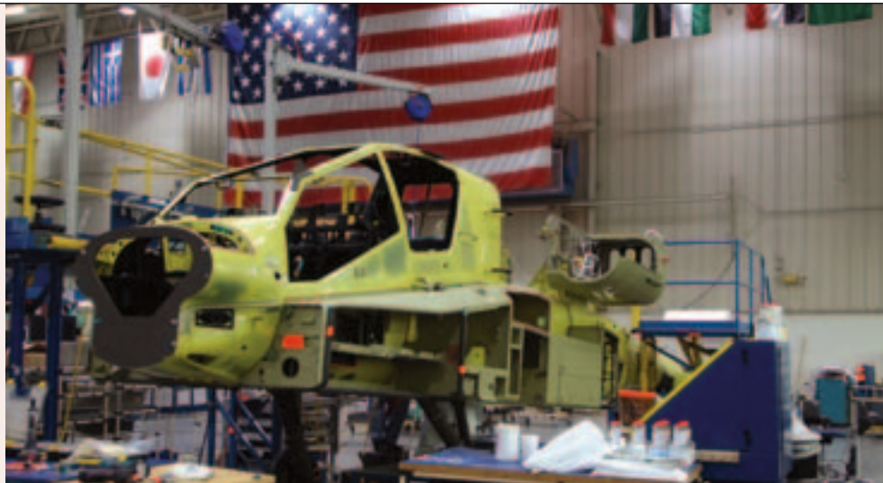
The Apache Longbow remanufacturing line converts older AH-64A Apaches into the AH-64D Longbow. The Boeing assembly line in Mesa, AZ, conducts this remanufacturing process. (Photo courtesy of Boeing.)
