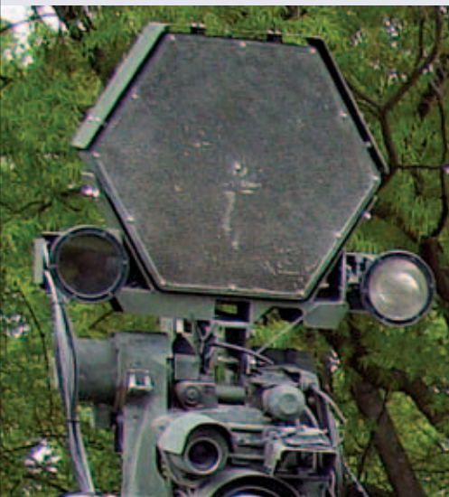
The rear nonlethal Remote Weapon Station was added to the Stryker ICV to support several FSEP components, including the long-range AHD, high-power white lights, and the 12-gauge shotgun. (U.S. Army photo.)
