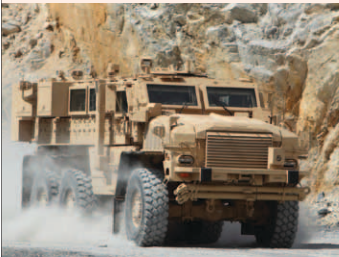
The Panther is a command and control vehicle that is also designed to neutralize or defeat explosive hazards. (U.S. Army photo.)
