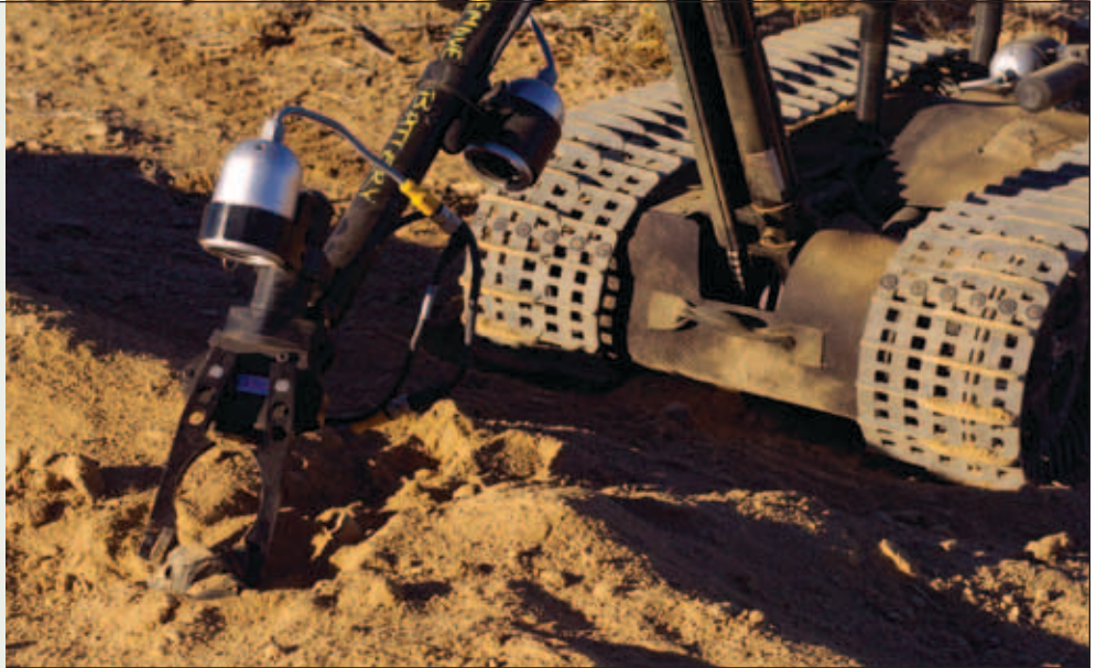
A Talon ordnance disposal robot prepares to unearth a simulated IED during an exercise. The Talon is an element of RS JPO's robotic system fleet. (U.S. Navy photo by MC3 Kenneth G. Takada.)
