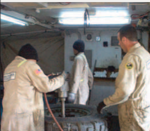
GDLS contractors at the FRA-I tire shop reassemble a Stryker wheel and tire assembly that will be put back into the forward supply system. (Photo by Lynden Lawson.)
