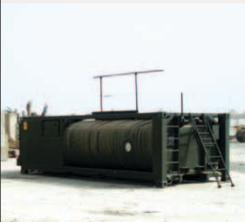
The 2,000-gallon Hippo water storage tank works with several of the Army’s water purification systems. (U.S. Army photo.)
