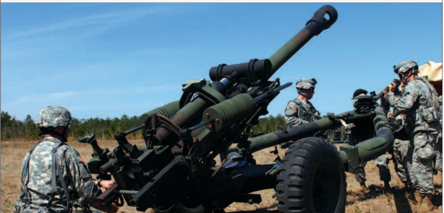
The DFCS capability is being integrated onto the 105mm M119A2 towed howitzer. Here, 1st Battalion, 258th FAR, New York ARNG Soldiers lift the back of an M119A2 howitzer to spin the cannon into firing position, March 8, 2010. (U.S. Army photo by SPC Ian Boudreau, 27th IBCT Public Affairs.)
