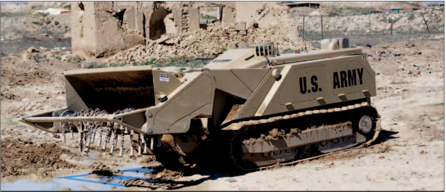
The RS JPO currently has one fully funded POR reflected in the FY10–15 POM for route clearance, which includes the M160 (MV-4B) Anti-Personnel Mine Clearing System seen here. (U.S. Army photo courtesy of RS JPO.)
