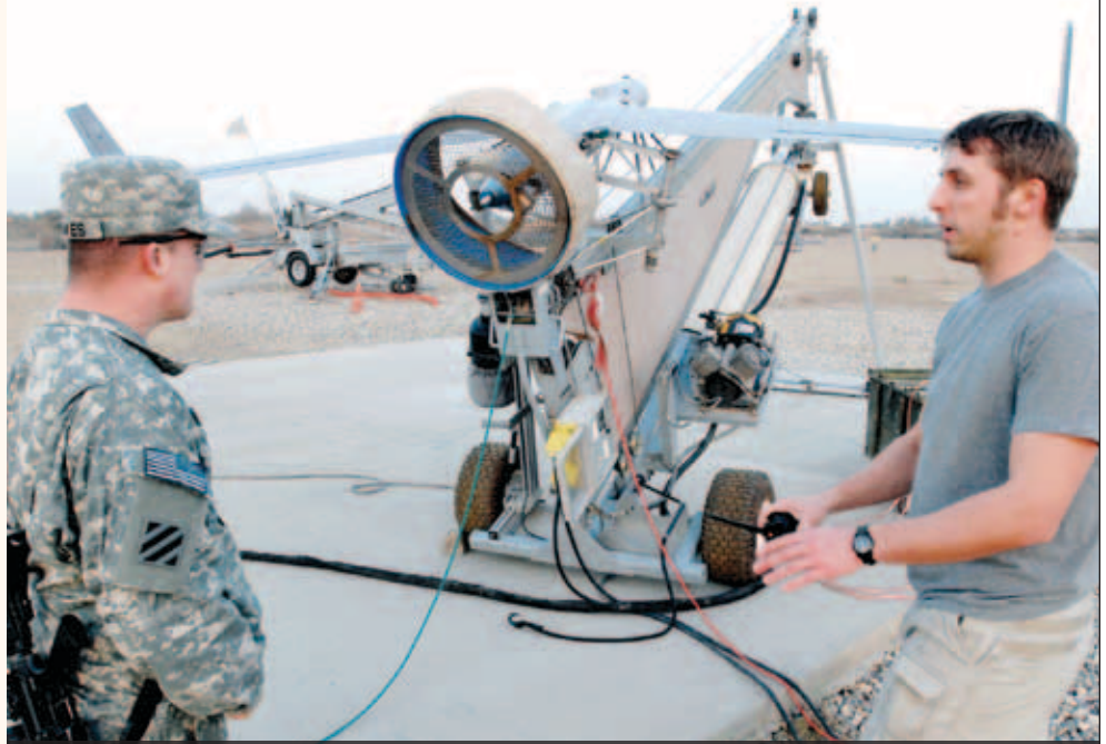
The AFSB's AL&T-D coordinates to ensure that FSRs assist in acceptance inspections and final issue of the equipment. Here, FSR Justin Fluegel explains the launch procedures for the ScanEagle Unmanned Aerial Vehicle to SGT Matthew Hayes, Headquarters Battery, 1-10 Field Artillery Battalion, at Forward Operating Base (FOB) Delta, Iraq. (U.S. Army photo by SSG Brien Vorhees.)
