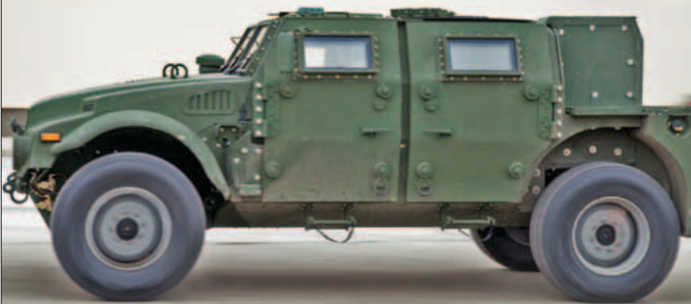
General Tactical Vehicles’ (GTVs) vehicle design provides an armored crew capsule with a V-shaped hull for protection against mines and improvised explosive devices, high-performance and off-road mobility, and deployability by land, sea, and air. (Photo by GTV.)
