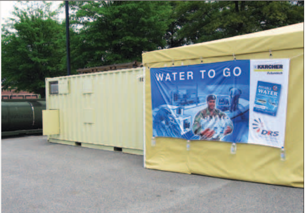
The EWPS can reliably produce 600–700 1-liter bottles per hour. In theater, the EWPS produces more than 500 bottles of water per hour and operates 6 days a week. (U.S. Army photo.)
