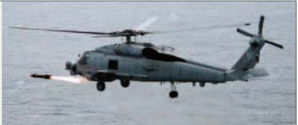
An SH-60B Sea Hawk helicopter assigned to the "Wolfpack" of Helicopter Anti-Submarine Squadron Light 45 launches an AGM-114B HELLFIRE missile at a small boat target. (U.S. Navy photo by Austin Long.)
