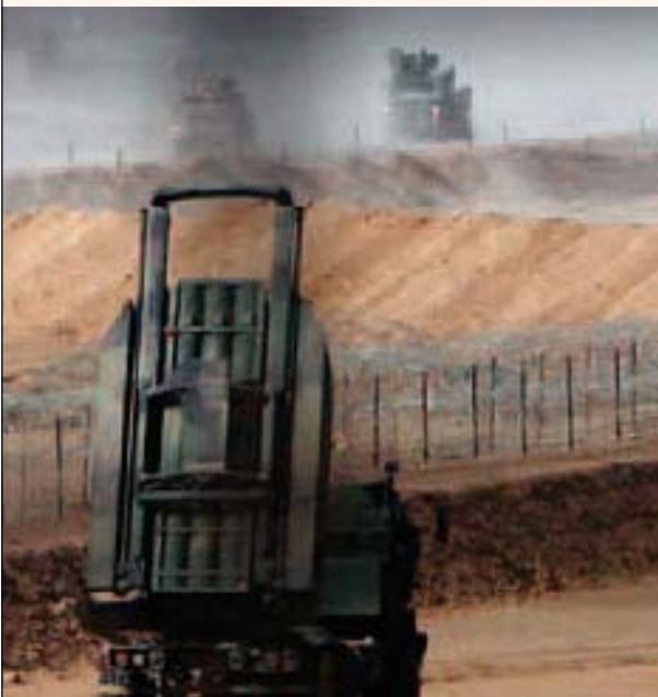
Marines with Btry D, 2nd Bn, 14th Marine Regt, set up a firing position in a HIMARS during a test fire at Camp Barber, Afghanistan, Feb. 15, 2009. HIMARS is able to launch its weapons and move away from the area at high speed before enemy forces can detect the launch site. (USMC photo by LCpl Ronald Stauffer, Special Purpose Marine Air Ground Task Force-Afghanistan.)
