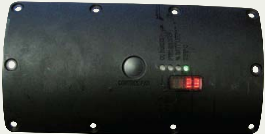
The HMU records the missile's power on time, captive carry time, ambient temperature, and battery life. In this photo, the temperature (23 C) is displayed. (U.S. Army photo by Deanie Blankinchip and Gloria Bell, JAMS Project Office Graphics Department.)
