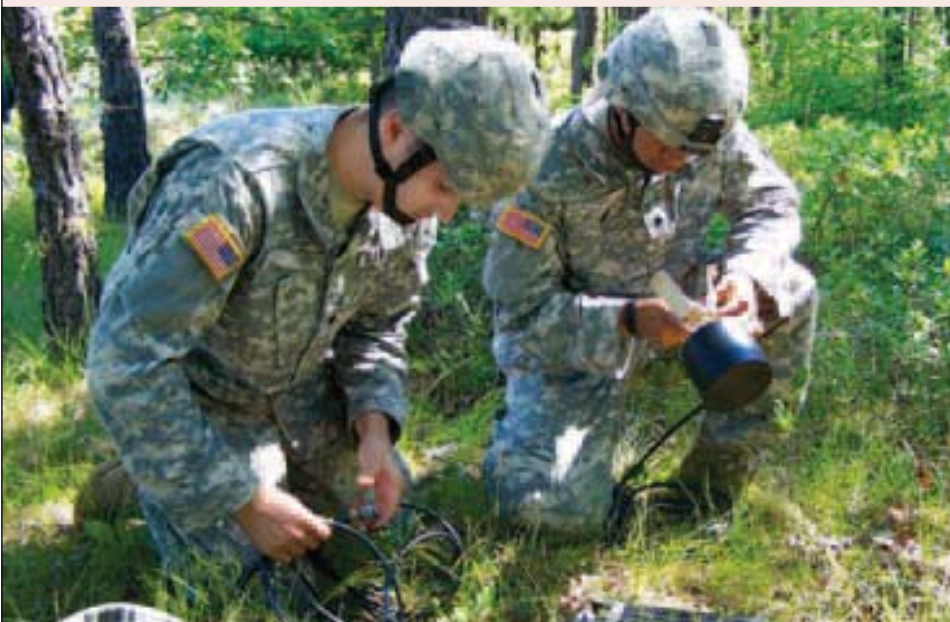
OSRVT is a mobile, lightweight, manpackable system that allows Soldiers to receive and display video and telemetry data, even while they are on the move, for enhanced SA. (U.S. Army photo courtesy of the UAS PO.)
