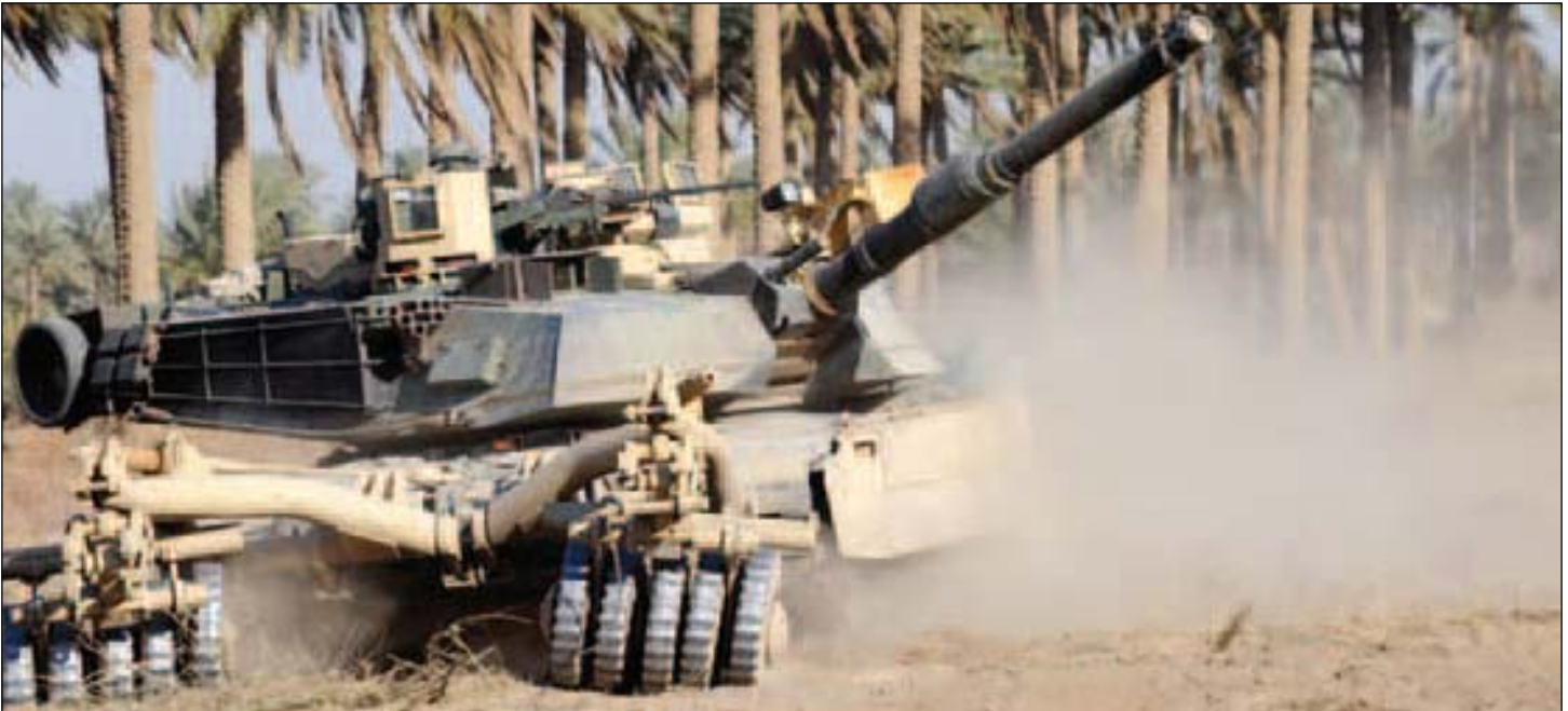
An M1A1 Abrams tank uses mine rollers to clear a palm grove of landmines in Iraq. Armored and tactical vehicles played crucial roles in penetrating, securing, and patrolling cities throughout Iraq and assisting in operational missions to keep warfighters safe. (U.S. Army photo by SPC Chase Kincaid.)
