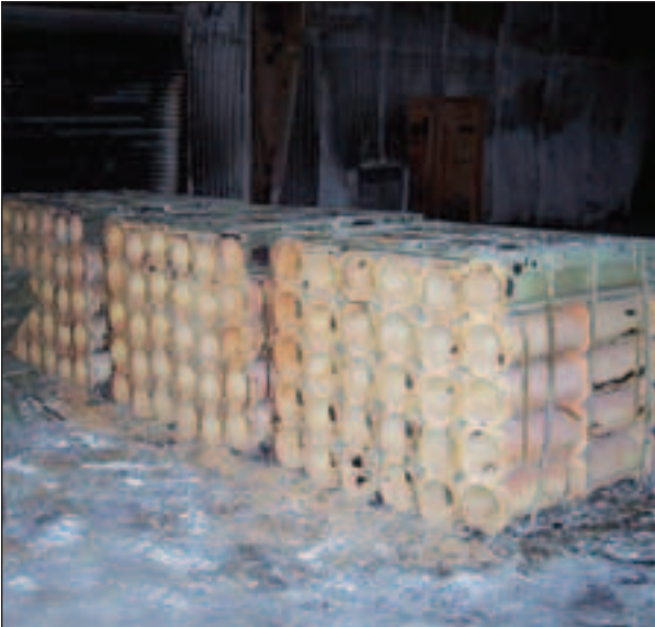
In a fire during the load/assemble/pack operations for the M232A1 Modular Artillery Charge System (MACS) at General Dynamics-Armaments and Technical Products, Camden, AR, the IM features of the MACS vented the pressure from the nearly 6,000 pounds of burning propellant housed in and around the building and prevented injuries to personnel. (Photo courtesy of Project Manager Combat Ammunition Systems, Picatinny Arsenal.)
