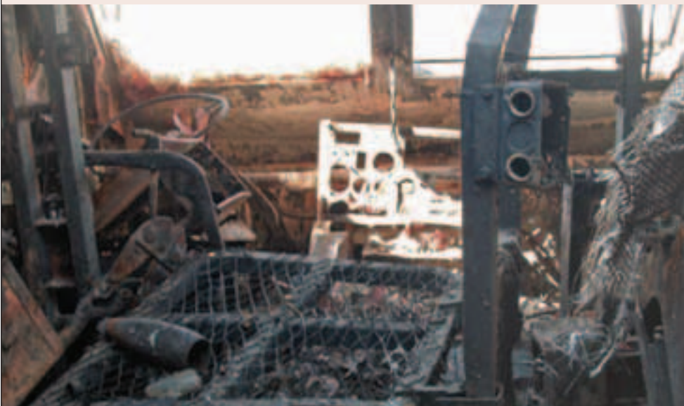
Shown here is the interior view of the MRAP in Ng's convoy after the Sept. 12, 2009, fire. An unexploded shell body from a M768 cartridge can be seen in the lower left. (Photo courtesy of PM CAS, Picatinny Arsenal.)
