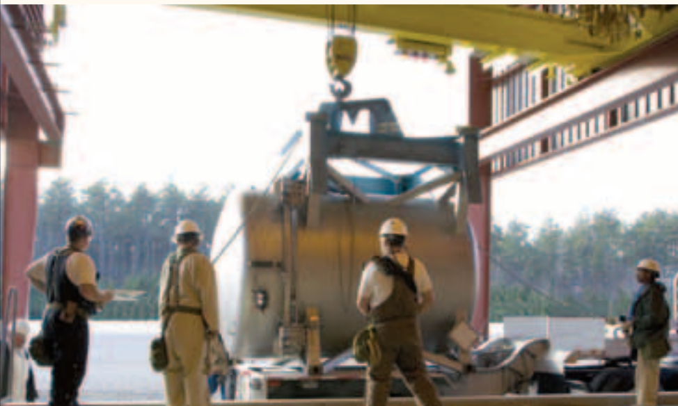
PBCDF munitions handlers watch the last Enhanced Onsite Container carrying VX M55 rockets being lifted by an overhead crane into the disposal facility’s container-handling building. (U.S. Army photo courtesy of CMA.)
