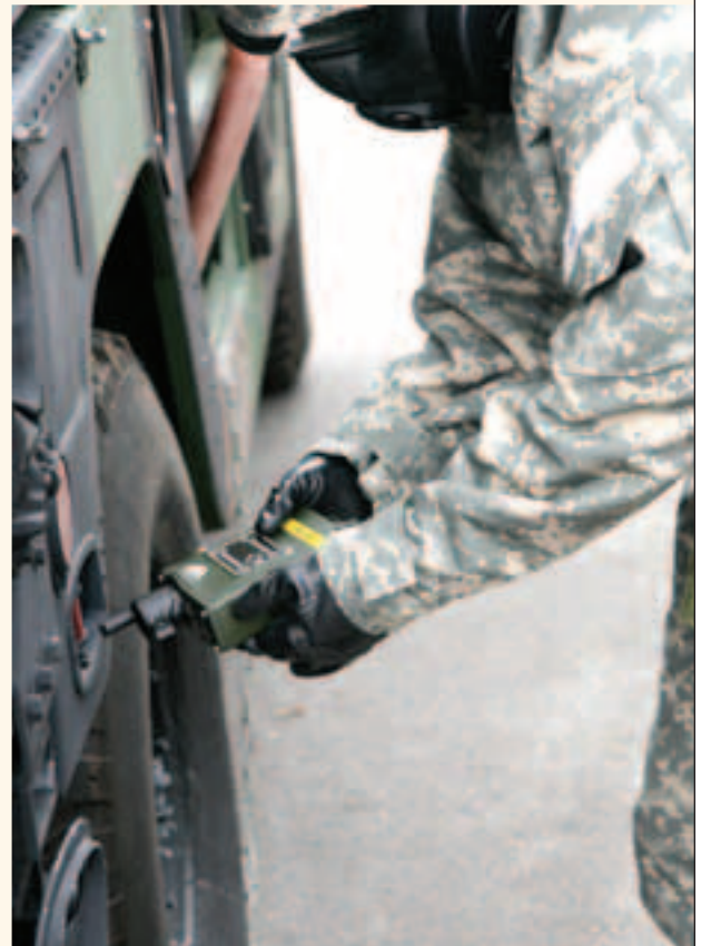
The JCAD is capable of detecting blood agents and toxic industrial chemicals, capabilities not seen in currently fielded hand-held detectors. Here, a Soldier dressed in Mission-Oriented Protection Posture gear surveys the surface of a vehicle with a JCAD. (U.S. Army photo.)
