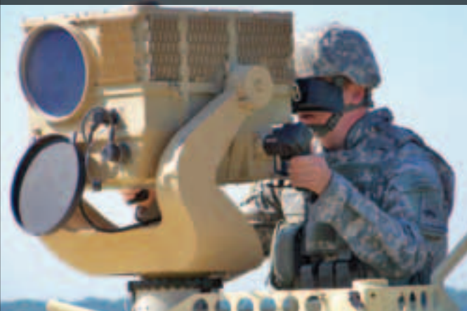
U.S. ground forces using the LRAS3 in conjunction with the JCIMS can verify friendly forces when targeting. (U.S. Army photo.)
