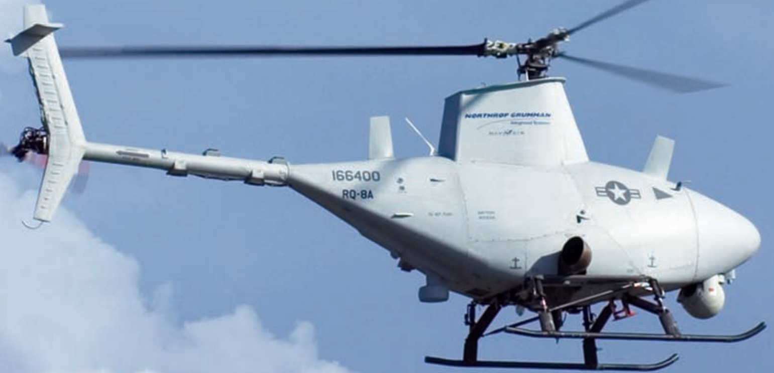
The Fire Scout will carry the TSP as well as STARLite, which will provide the future system with SAR/GMTI. (Photo courtesy of PM FCS.)
