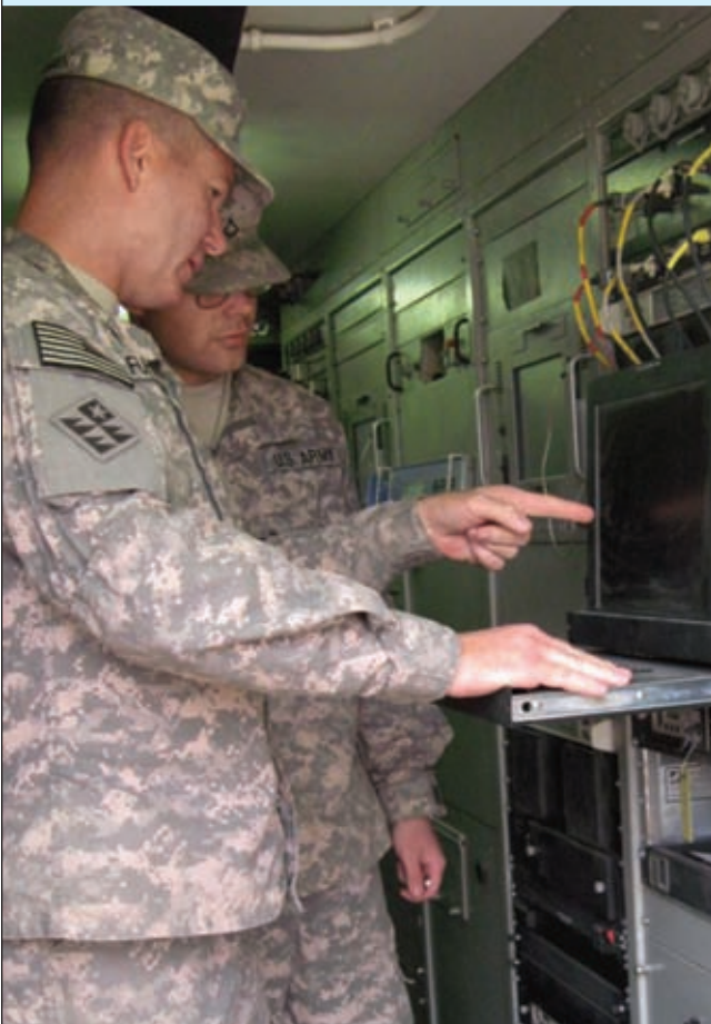
SSG Guy Fuhrman shows PFC Joshua Smith the operation of the orderwire in an AN/TSC-85D TACSAT at Camp Victory, Iraq. (Photo by Donald W. Mumma, CECOM Senior Command Representative, U.S. Army Sustainment Command Headquarters.)
