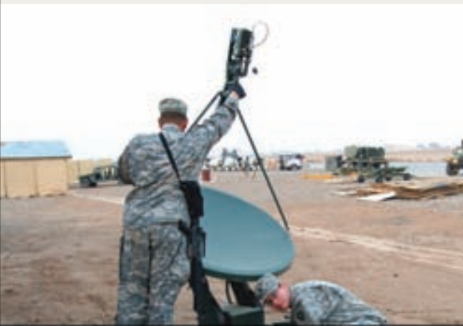
SSG Stephen Achee and SSG Elizabeth Engstedt, Combat Service Support (CSS) Automated Management Office, Headquarters Support Co., 449th Aviation Support Battalion, Texas Army National Guard, maintain the CSS Very Small Aperture Terminal satellite at Logistical Support Area Anaconda, Baghdad Province, Iraq. (U.S. Army photo by SGT Huey Kehl.)
