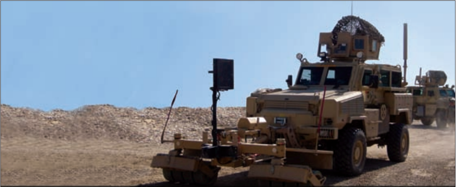
TARDEC has fielded more than 360 SPARKs to Soldiers in the GWOT. The SPARK provides additional stand-off capability to vehicles and crews against pressure-activated improvised explosive devices. (U.S. Army photo courtesy of TARDEC.)
