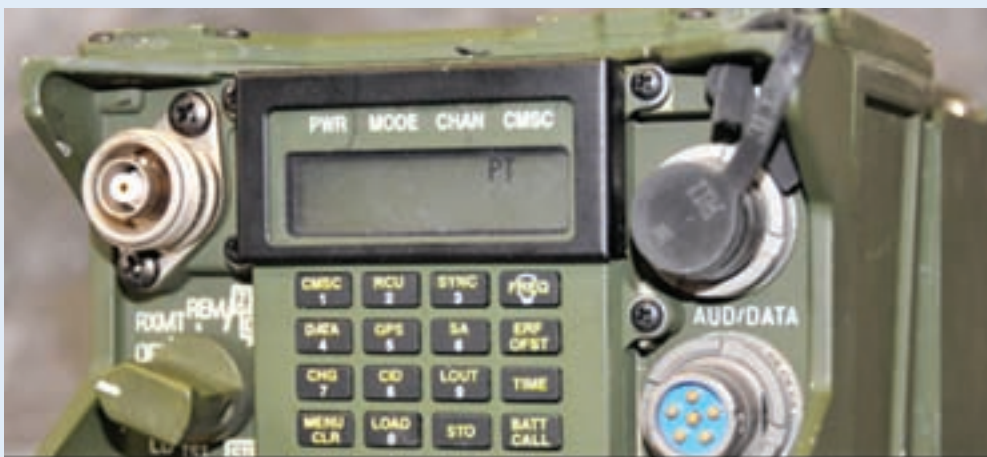
The Advanced System Improvement Program version of the Single-Channel Ground and Airborne Radio System is being fielded to the Army and has an inventory of nearly 300,000. (U.S. Army photo by Jason Bock.)
