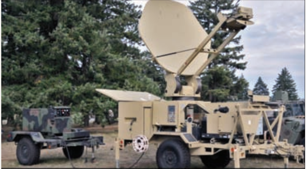
A WIN-T Increment One STT is powered by one trailer-mounted Tactical Quiet Generator. (U.S. Army photo by Jason Bock.)
