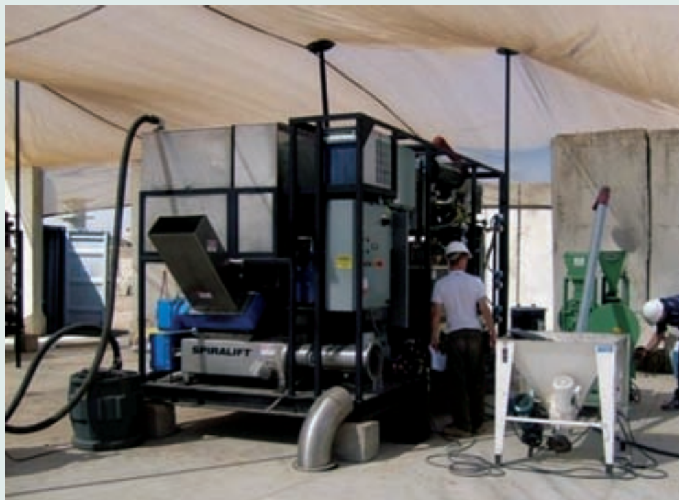
The Army is exploring the capability of converting garbage to energy with the TGER, a system already being tested in theater. Here, contractors install a TGER at Camp Victory, Iraq. (U.S. Army photo by Jerry Warner, Defense Life Sciences.)
