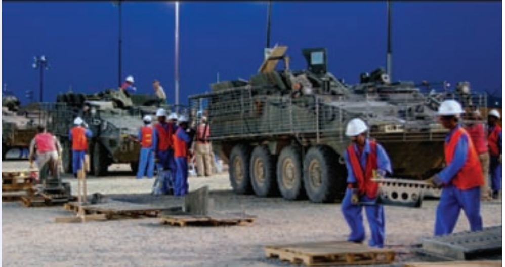
Contract workers with General Dynamics Land Systems work under the lights to remove slat armor from 4th Stryker Brigade Combat Team, 2nd Infantry Division, Stryker Combat Vehicles, at a 401st AFSB work area at Camp Arifjan, Kuwait. (U.S. Army Photo by Jim Hinnant, 401st Army Field Support Brigade.)
