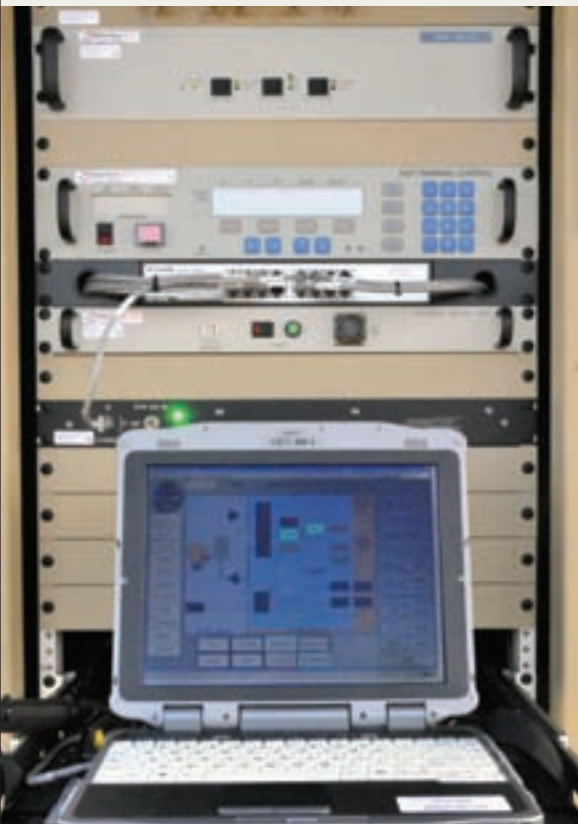
The WIN-T Increment One STT can be configured to operate over Ku- or Ka-band satellite frequencies. (U.S. Army photo by Jason Bock.)
