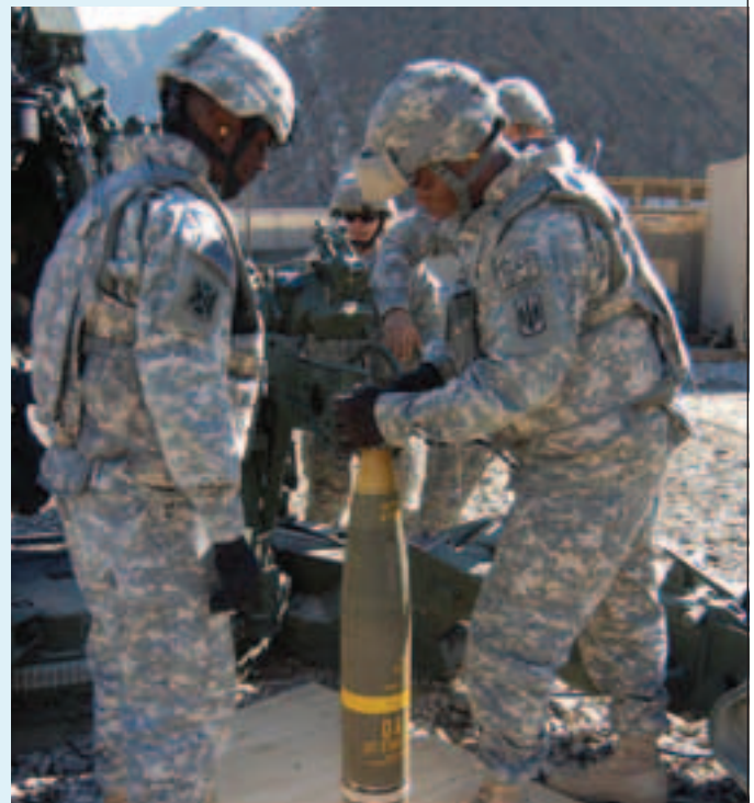
SSG Darius Scott (left) watches SSG Jamare Cousar, Charlie Co., 3rd Bn, 321st FAR, use the Enhanced Portable Inductive Artillery Fuze Setter to program the proper grid coordinates into the Army's new GPS-guided Excalibur round before the very first fire of the round in Afghanistan at Camp Blessing, Feb. 25, 2008. (U.S. Army photo.)
