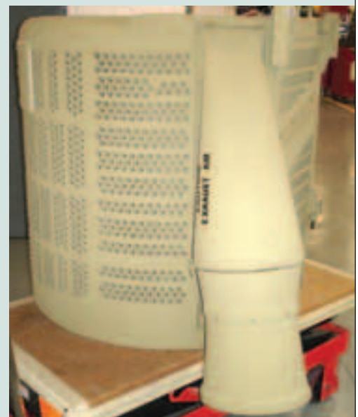
The EAPS is an FCT program success story. When used on helicopters flying in dusty or sandy environments, the EAPS can significantly increase engine life because it decreases erosion of engine components. (U.S. Army photo.)
