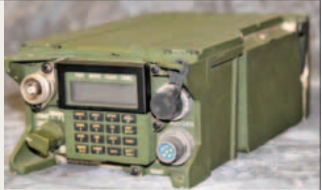
Shown here is PEO C3T's Single Channel Ground and Airborne Radio System advanced system improvement program radio, the primary voice control radio for Soldiers at battalion level and below. (U.S. Army photo by Jason Bock.)
