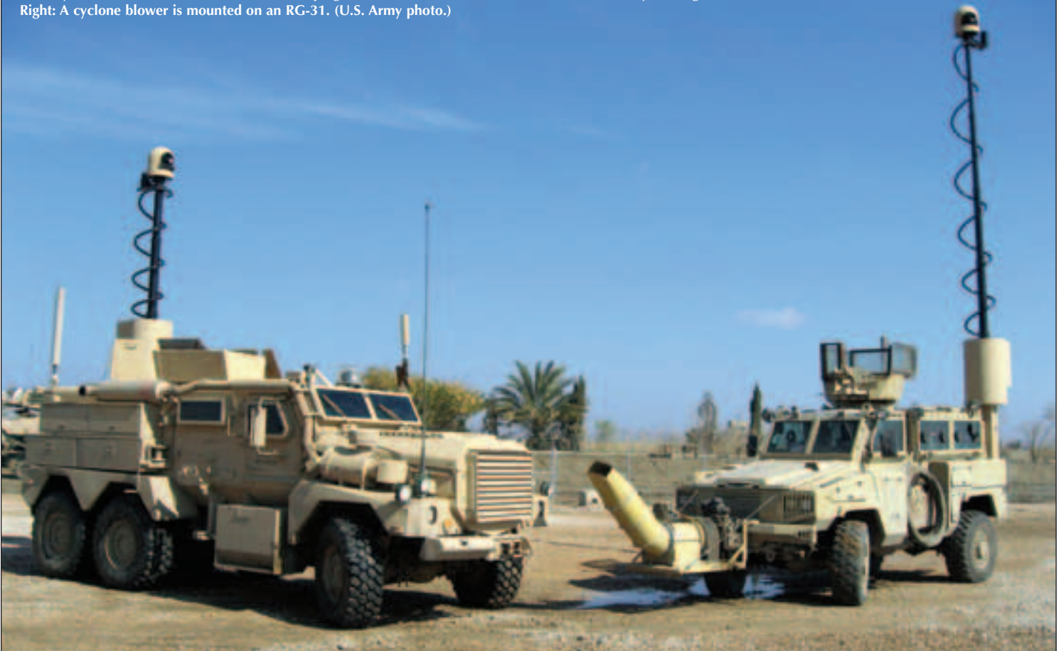
Left: Gyro-stabilized cameras and a 25' telescoping mast allow detection of IEDs on the move in day and night conditions. Right: A cyclone blower is mounted on an RG-31. (U.S. Army photo.)
