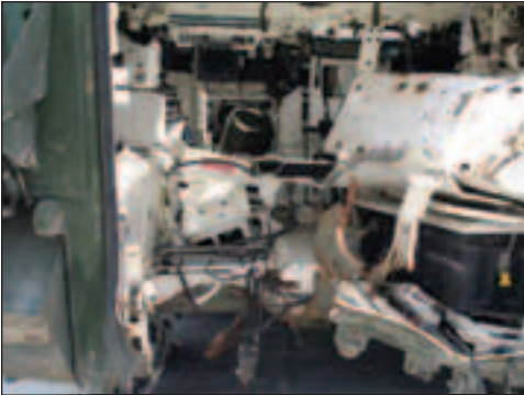
Before BDR: Stryker damaged by an IED. (Photos by Tim Armstrong, GDLS Qatar.)
