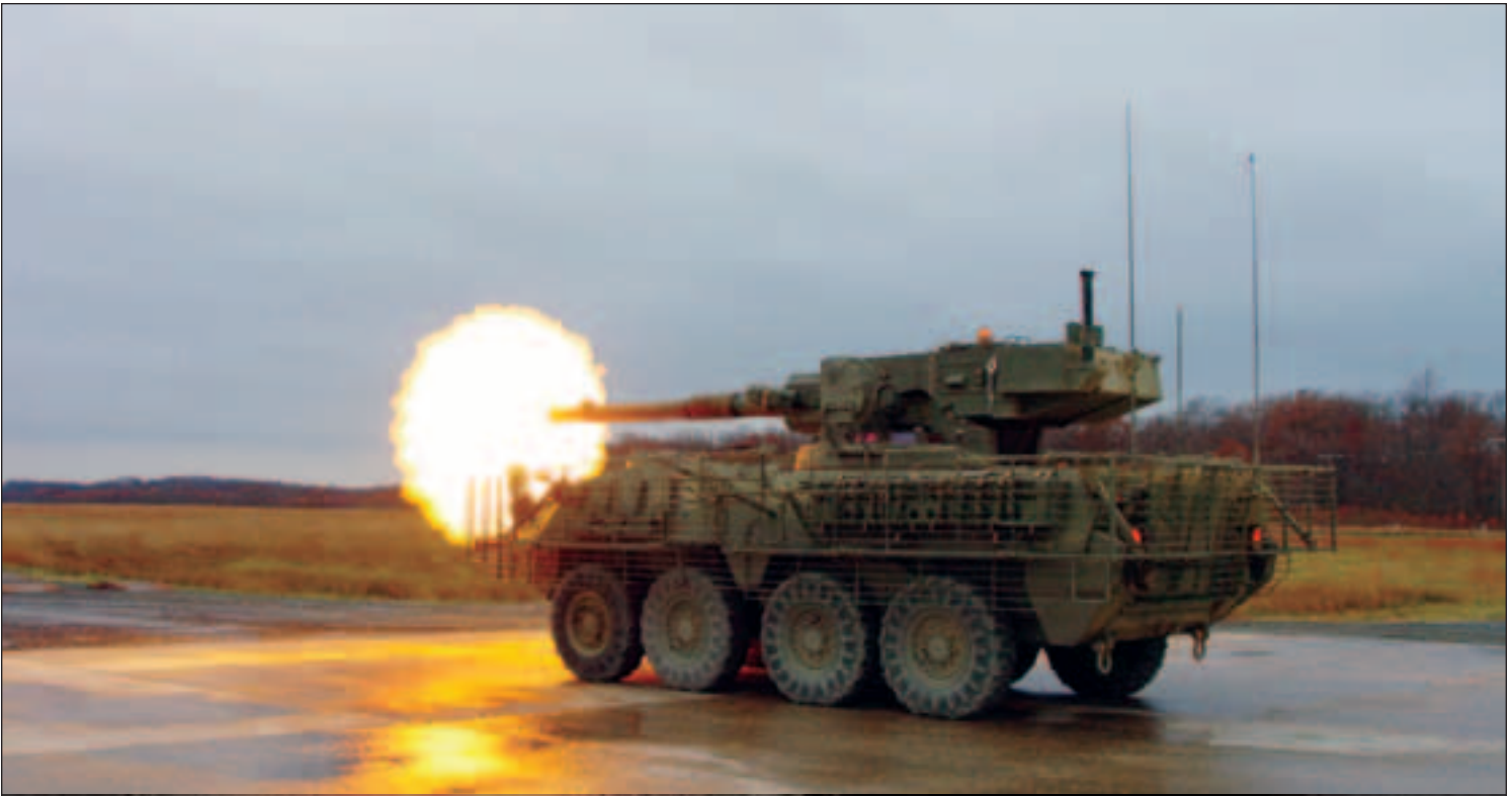
The Stryker MGS undergoes a live-fire test at ATC. The ATC is one of ATEC's test centers across the U.S. that conducted ballistic, mobility, and survivability testing on Stryker MGS prior to its deployment into theater. (Photo courtesy of ATC.)
