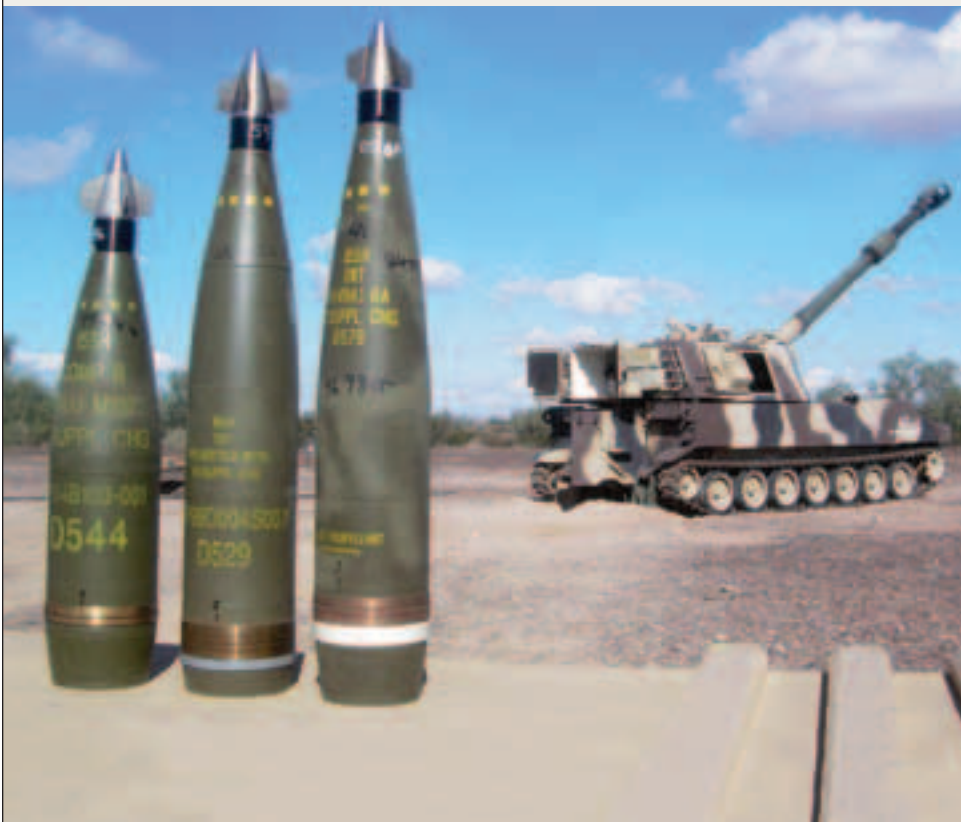
The PGK increases cannon artillery accuracy by tracking the projectile position location and determining trajectory navigation solutions. This results in improved accuracy, quicker target kills, less collateral damage, and reduced logistics burden. (U.S. Army photo.)
