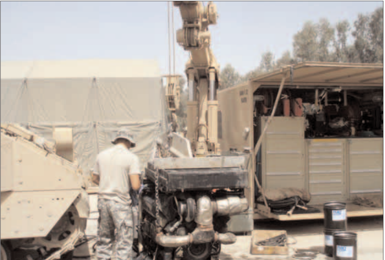
PM JCSS focuses on persistent combat and provides capabilities necessary for Expeditionary Forces. Here, a Soldier uses the Forward Repair System in the AOR to remove a power pack. (Photo courtesy of PEO CS&CSS.)
