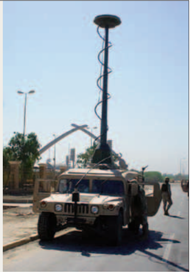
Here, a Prophet vehicle stands with its mast extended in the streets of Baghdad. (U.S. Army photo courtesy of PEO IEW&S.)
