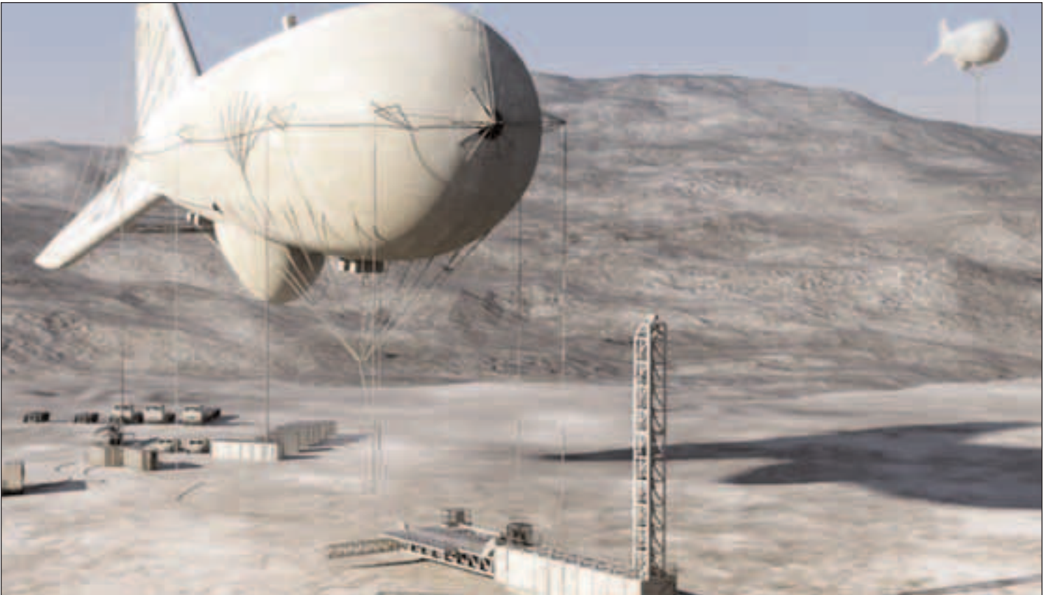
JLENS, a tethered aerostat, can stay aloft up to 30 days providing 24-hour radar coverage for long-range surveillance and fire control sensor capabilities. Here, JLENS is attached to the ground station. (Artist rendering courtesy of PEO MS.)
