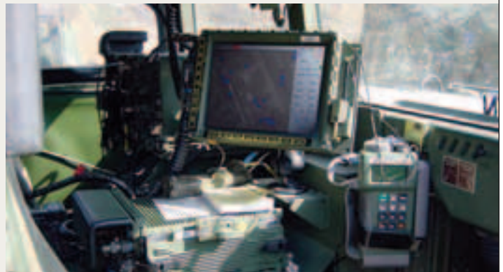
PEO C3T's FBCB2-BFT, shown here, provides a graphical representation of friendly vehicles and aircraft on a topographical map or satellite image of the ground. (U.S. Army photo.)
