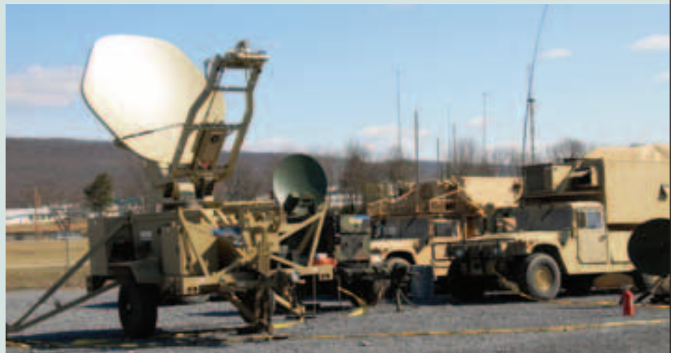
A WIN-T Increment 1 KU trailer is shown during Operation TOCFEST . (U.S. Army photo by Richard Mattox, PEO C3T.)
