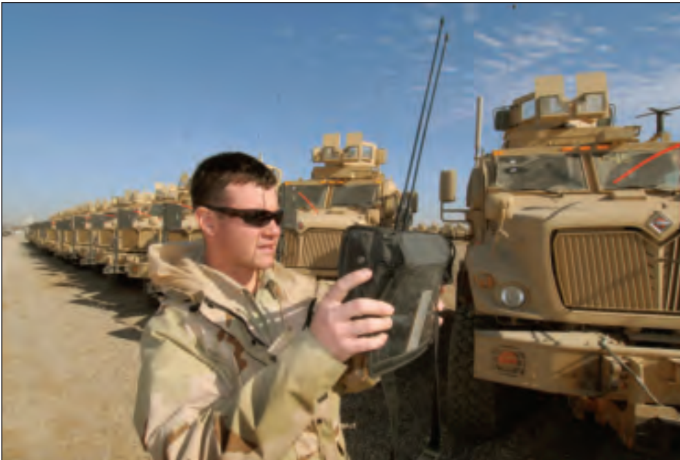
The CTSF SE&I department supports engineering assessments on new and developing C4I products. Here, Army civilian Paul Vanlucvender, an electronics integrated systems mechanic in the Command, Control, and Computers Avionics Directorate, performs operational verification of electronics systems on a Mine Resistant Ambush Protected vehicle in Southwest Asia in March 2008. (U.S. Army photo by Steve Grzedzinski.)
