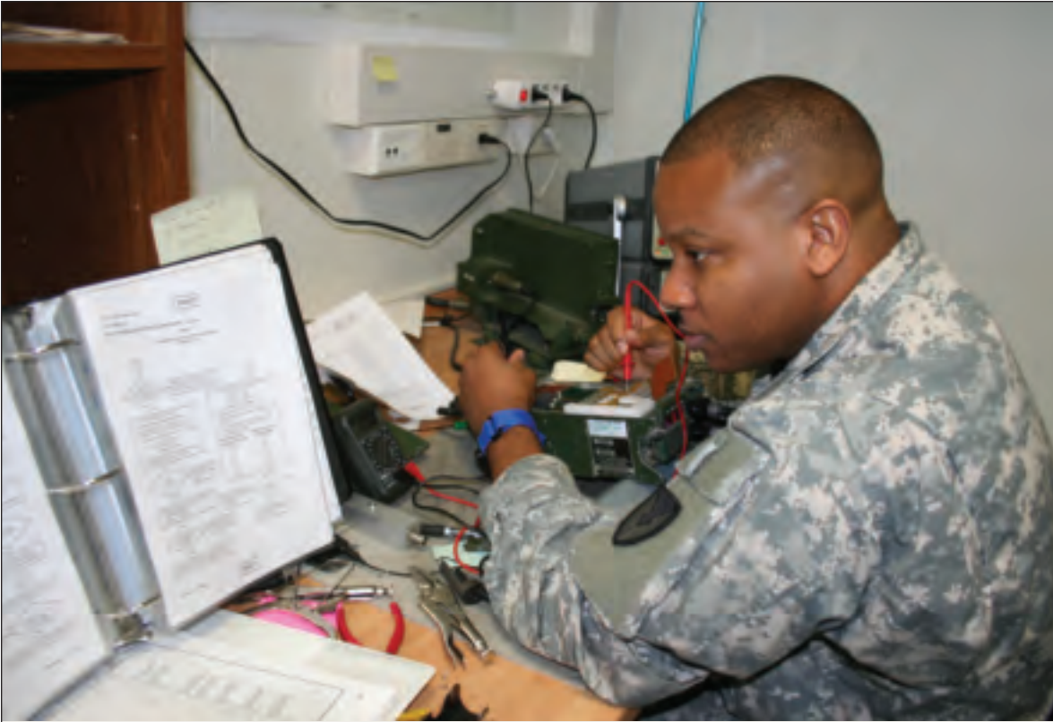
AFSBs leverage reachback capabilities to provide AL&T technical and call-forward support from the national sustainment base. Here, SSG Thomas Alexander, the noncommissioned officer-in-charge for the 3rd Battalion, 405th AFSB radio and communications security shop, Livorno, Italy, performs a quality assurance test on electronic gear while deployed to the Vicenza, Italy, Installation Materiel Maintenance Activity. (U.S. Army photo by Giovanni Comiati.)
