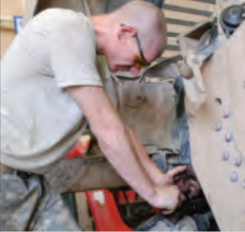
SPC Micah Mead, a tracked vehicle mechanic, replaces the ball joint on an up-armored HMMWV at Camp Virginia, Kuwait. (U.S. Army photo by SGM Richard Greene.)
