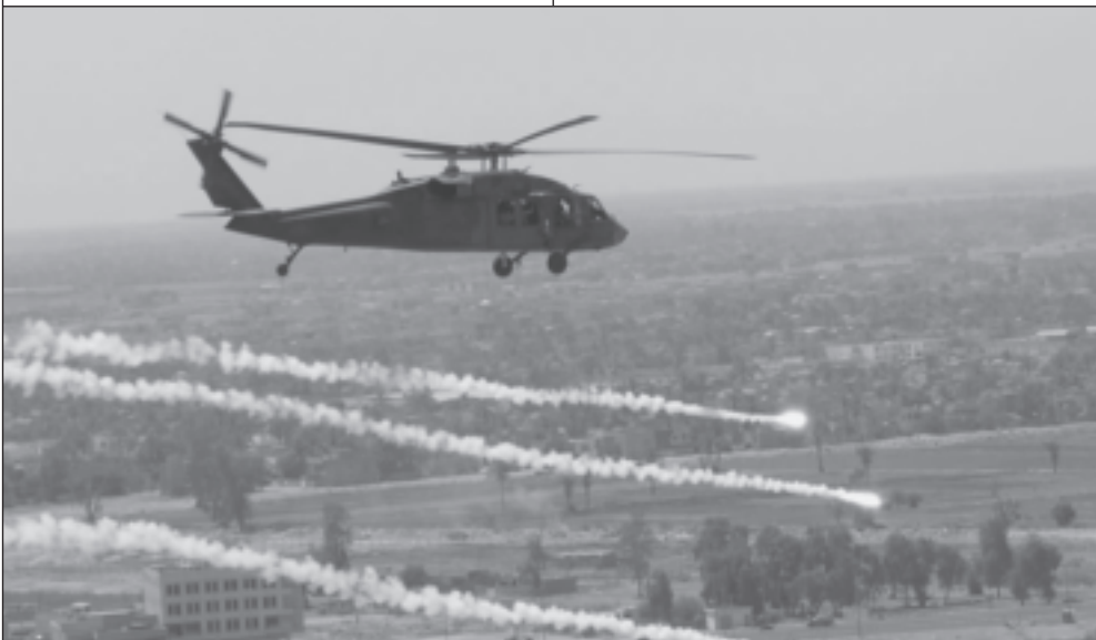
A UH-60 Black Hawk helicopter fires flares during a combat troop insertion during OIF. Transport helicopters are especially vulnerable to shoulder-fired IR-guided missiles. The new LA59 flare will greatly improve crew survivability in both Army fixed- and rotary-wing aircraft. (U.S. Army photo courtesy of PM CCS.)
