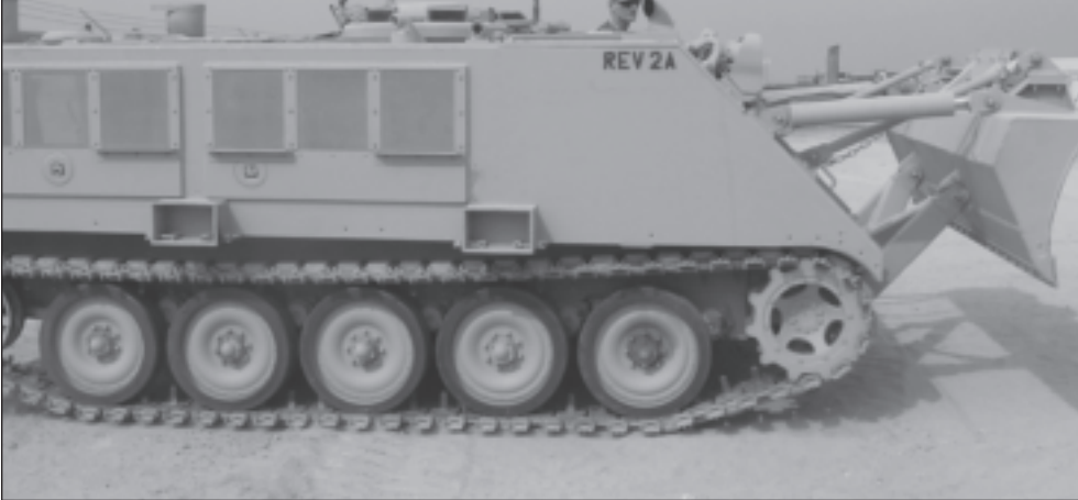
The M113A2 APC REV is designed to increase Soldier survivability during peacekeeping, low-intensity conflict and crowd control situations. REV features include six modular crowd control munitions, modified firing ports and improved SA. (U.S. Army photo courtesy of ARDEC.)
