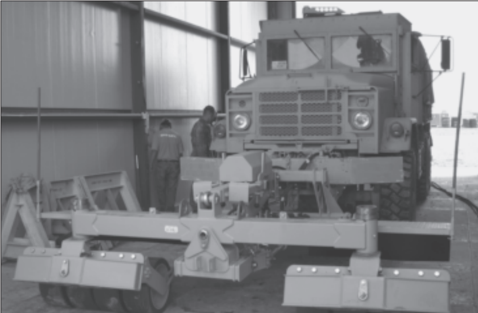
Here, technicians finish outfitting an M900 5-ton truck series with SPARK at an FOB in Iraq. The rollers are designed to defeat pressure-sensitive triggered IEDs by forcing the blast down and away from the vehicle. (U.S. Army photo.)
