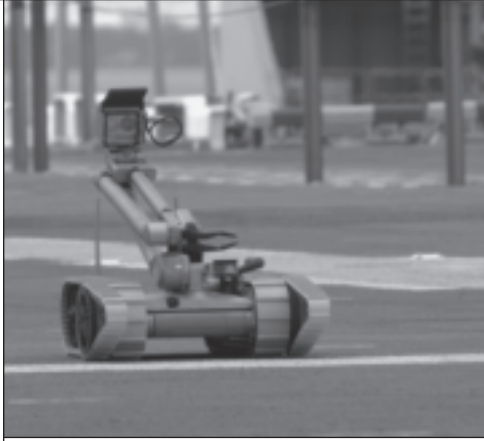
A PackBot remote-controlled robot from the U.S. Navy (USN) Explosive Ordnance Mobile Unit 2 is put through its paces during an IED drill aboard the Wasp Class Amphibious Assault Ship USS Bataan (LHD 5). (USN photo by MC2 Elizabeth R. Allen.)
