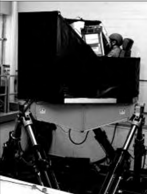
A participant operates the CAT mounted on the RMS during a recent experiment. TARDEC and ARL use the simulator to test issues including the effects of ground vehicle motion environments on Soldier performance. For illustration purposes, the crew station is opened. However, for testing purposes, the crew station can be enclosed to simulate a "buttoned-up" environment. (Photo courtesy of TARDEC.)
