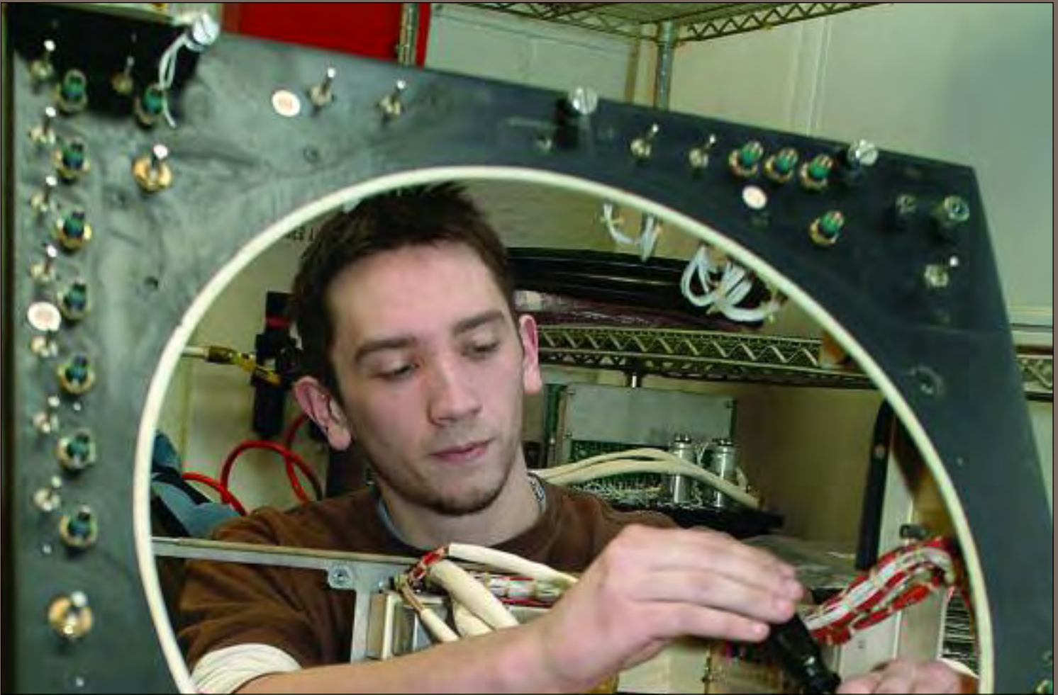
TYAD Electronics Technician Steveland McAllister prepares a planned position indicator for mechanical inspection prior to testing and installation into an AN/TPS-75. The indicator is a visual interface between the system and the technician, allowing 360-degree surveillance of the sky. The radar system is a mobile, tactical radar system capable of providing long-range radar azimuth, range and height information along with IFF capability for operations and control of tactical aircraft. (U.S. Army photo courtesy of TYAD.)
