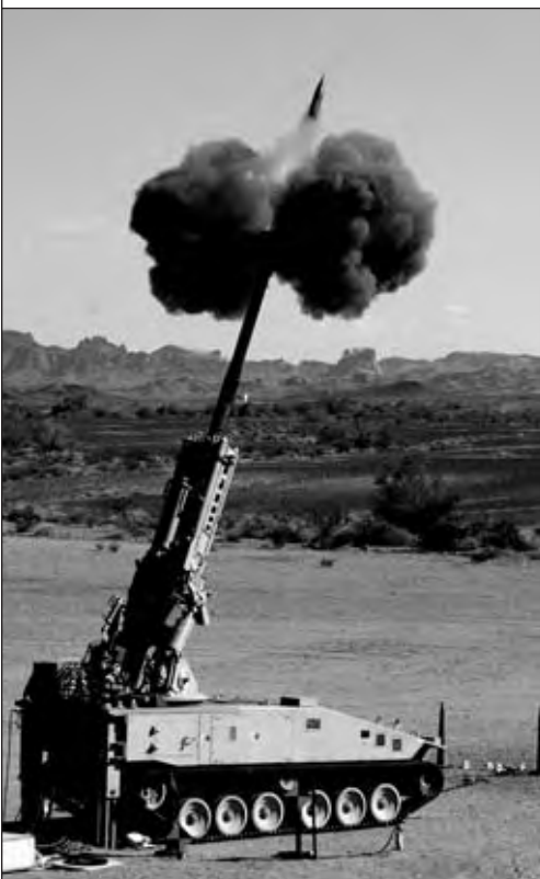
Here, an NLOS-C test platform fires a round last year at a test range at YPG. Likewise, successful firing of Excalibur at YPG has resulted in a CEP of less than 10 meters at all ranges. (Photo courtesy of the YPG Public Affairs Office.)
