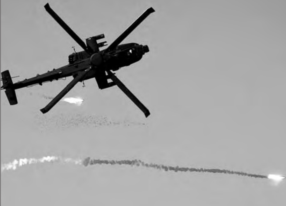
An AH-64 Apache helicopter ATTC XP crew conducts mission-focused CMWS flare separation testing in September 2005. (ATTC photo by Paul Reynolds.)
