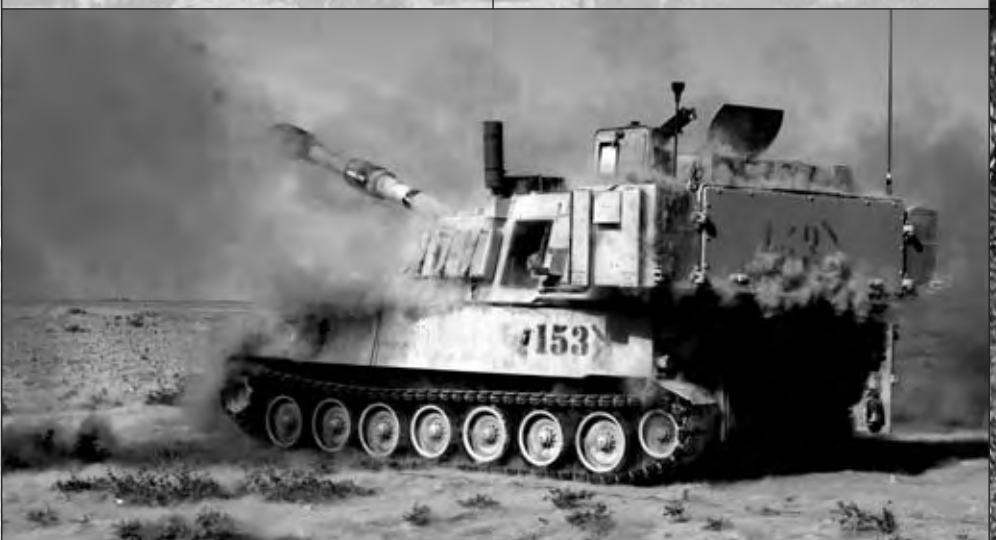
Soldiers from A Battery, 3rd Battalion, 29th Field Artillery Regiment, 3rd BCT, 4th Infantry Division (4ID), fire their M109A6 Paladin 155mm Self-Propelled Howitzer during an operational mission in support of Operation Iraqi Freedom (OIF). (U.S. Army photo by SGT Jack Morse, 982nd Signal Co. (Combat Camera).)
