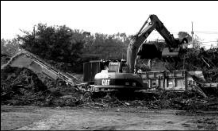
Woody debris is collected and turned into mulch at a USACE-contracted debris collection site in the aftermath of Hurricane Katrina. (USACE photo by George Stringham, St. Louis (MO) District Public Affairs Office.)
