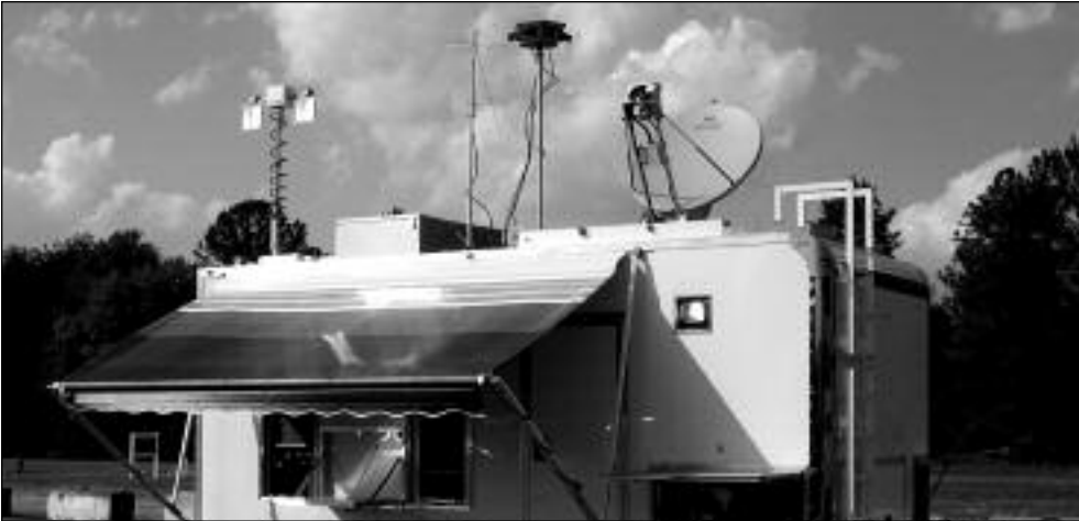
Radio communications was one of the NGB's biggest challenges during the disaster relief response to the Gulf Coast region's devastating hurricane season last year. The Guard's goal for this hurricane season is to pre-position communications equipment like the trailer pictured here. This self-contained, mounted incident site emergency communications system features voice, data, video and satellite reach-back capability, allowing NGB personnel to communicate with state and local authorities and fire, military and law enforcement agencies. Four trailers have been ordered off of a direct award contract valued at $1.8 million. (Photo courtesy of NGB Public Affairs.)
