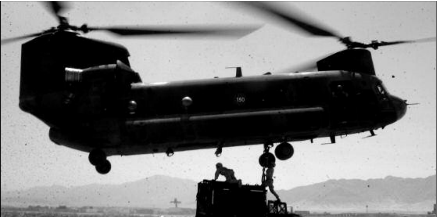
AMC's focus on logistics enablers — enhanced deployment, reduced logistics footprint and reduced logistics costs — ensures that the operational Army will always have the equipment and supplies it needs, when and where Soldiers need it most. Here, Soldiers sling load a Humvee to a CH-47 Chinook helicopter during an operation near Bagram, Afghanistan. The Soldiers are assigned to the 25th Infantry Division (Light), supporting the Joint Logistics Command during Operation Enduring Freedom. (U.S. Army photo by SFC Sandra Watkins Keough.)
