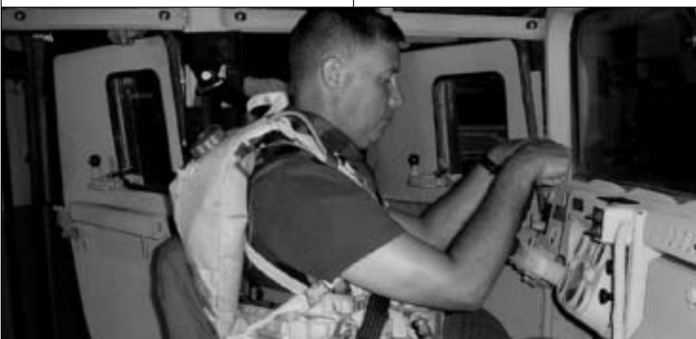
The new seat restraints offer ease of ingress and egress and fit 95 percent of males wearing Interceptor Body Armor and combat gear. (U.S. Army photo courtesy of PM TV.)
