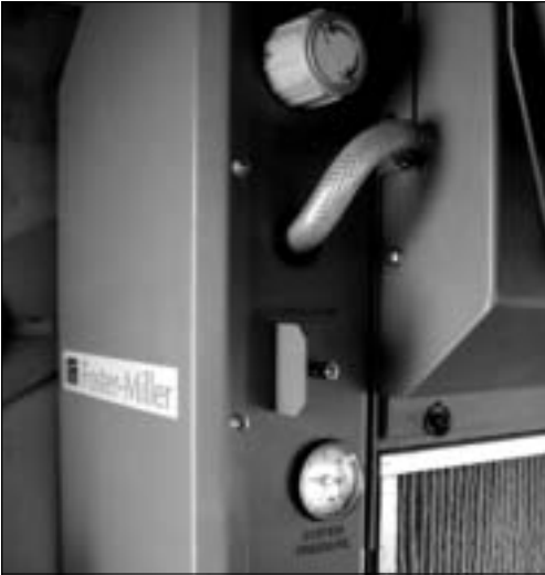
The water-filled vests fit under a Soldier's normal body armor and are connected via hoses to the vehicle's MCC subsystem. The chilled water is circulated through the garment. (U.S. Army photo courtesy of TARDEC.)
