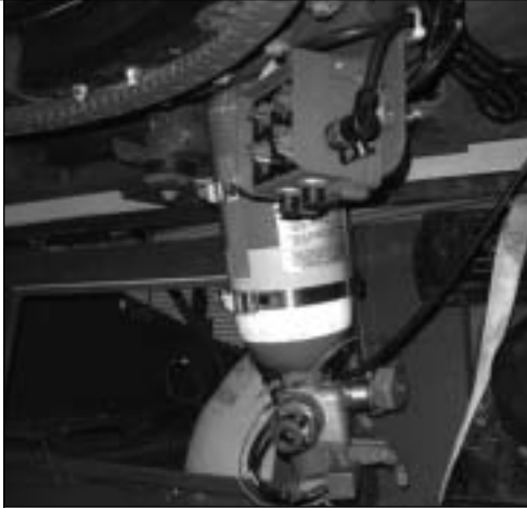
PM TV and TARDEC are leveraging current Army technologies to tailor a mounted fire suppression system for the M1114 Humvee. (U.S. Army photo courtesy of PM TV.)
