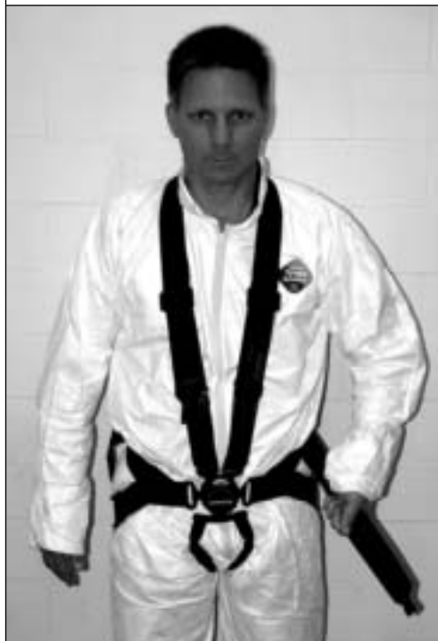
The gunner's restraint system is a quick-response solution that is designed to keep the gunner inside the vehicle in the event of a rollover or collision-avoidance event. (U.S. Army photo courtesy of PM TV.)
