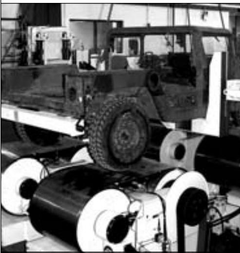
ATC's Roadway Simulator is the largest facility of its kind in the United States. It will play a significant role in testing the Army's FCS components. (Photo courtesy of ATC.)
