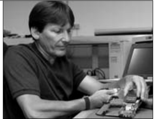
Mark Cooper inserts a microprocessor chip into the mother board of an Itronix® laptop computer at Tobyhanna Army Depot. Tobyhanna and 30 Forward Repair Activities worldwide now repair computers under a manufacturers’ warranty repair program. (U.S. Army photo.)
