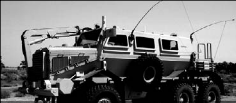
This 24-ton Buffalo vehicle offers combat engineers a safe, effective means of searching for IEDs by using its 30-foot remote-controlled hydraulic arm to prod suspicious items found along roadways and main supply routes. Innovations such as this are saving Soldiers' lives and thwarting the insurgency's best efforts. (U.S. Army photo by MSG Lek Mateo.)
