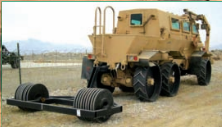
The Buffalo can also be equipped with attachments, such as this roller array. (Photo courtesy of PEO Ammunition.)
