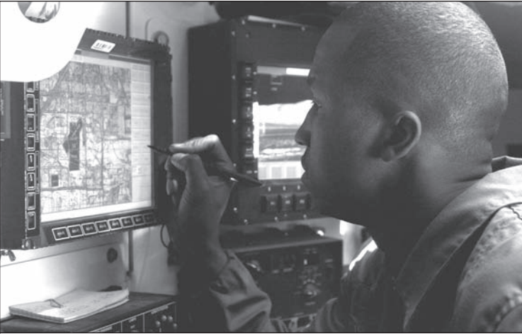
SFC Kenneth R. Dawson checks the map on his Force XXI Battle Command Brigade and Below display during a live-fire training exercise at the National Training Center, Fort Irwin, CA. Present tactical wireless networks experience degraded network performance as network demands increase. CERDEC has developed an adaptive application middleware that will dynamically control what the application offers to the network based on the network's health at any given point in time. (U.S. Army photo by CPT Tim Beninato, 28th Public Affairs Detachment.)
