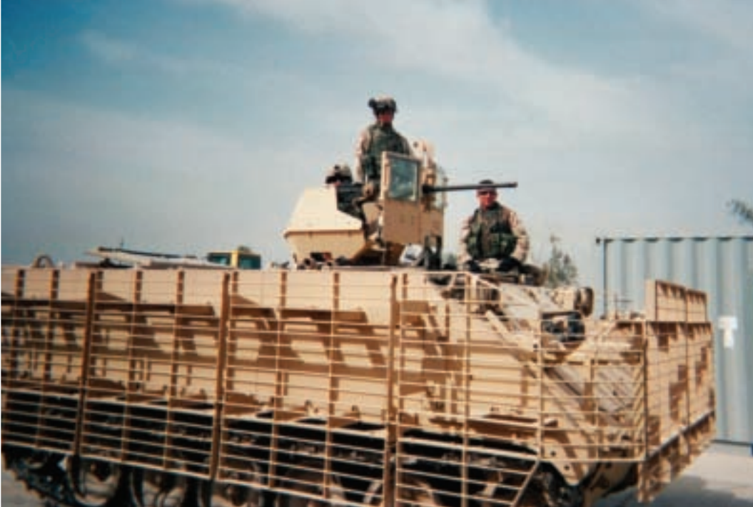
M-113 armored personnel carrier equipped with add-on armor. (U.S. Army photo courtesy of Project Manager Combat Systems.)
