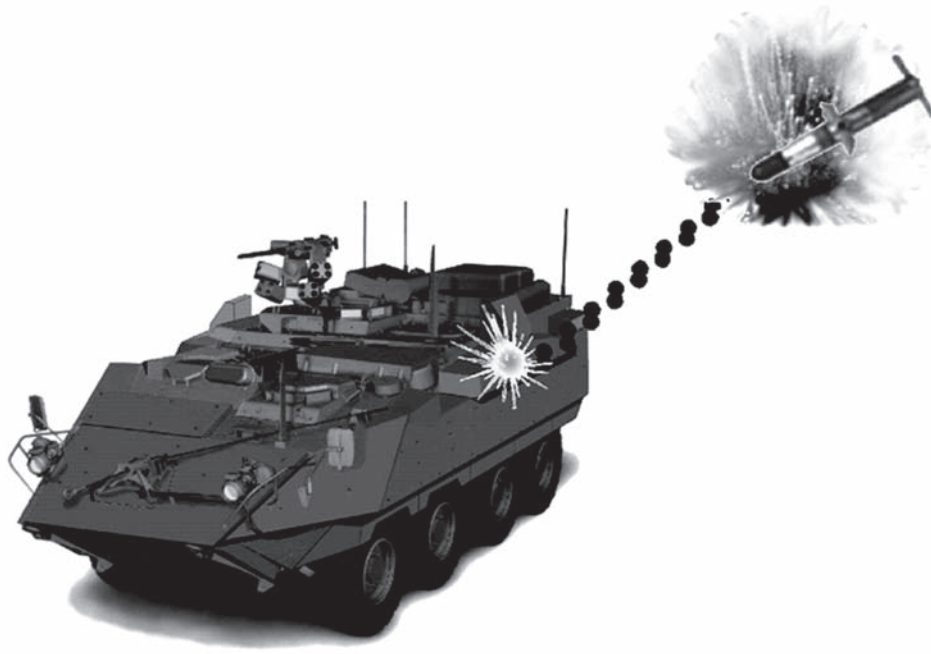
Figure 1. An APS-deployed countermeasure intercepts an incoming missile.
