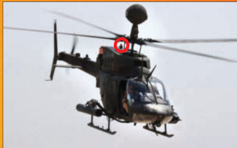
An IR strobe shown circled in red. (U.S. Army photo by Albert Eaddy.)
