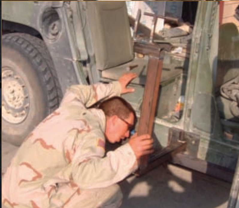
SAW gun vehicular mounts are one of the critical things manufactured by the MPHs. (Photo courtesy of TARDEC.)
