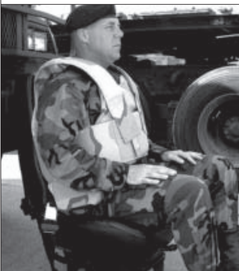
V-BASS, initially designed for the M915 FoV, protects truck crews from small-arms fire and IED fragments. (U.S. Army photo.)
