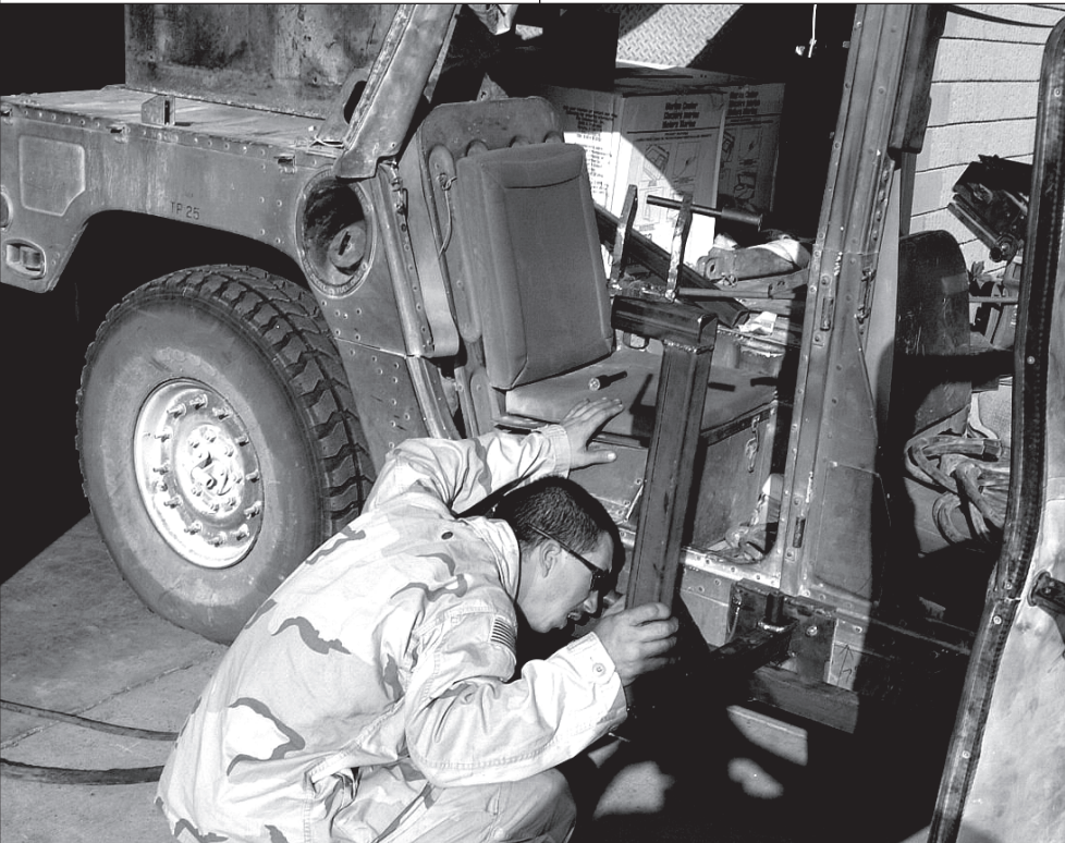
SSG Kenneth Kennedy inspects a modified gun mount that the LMM produced, which he installed and welded in place. (U.S. Army photo by Greg Outland.)
