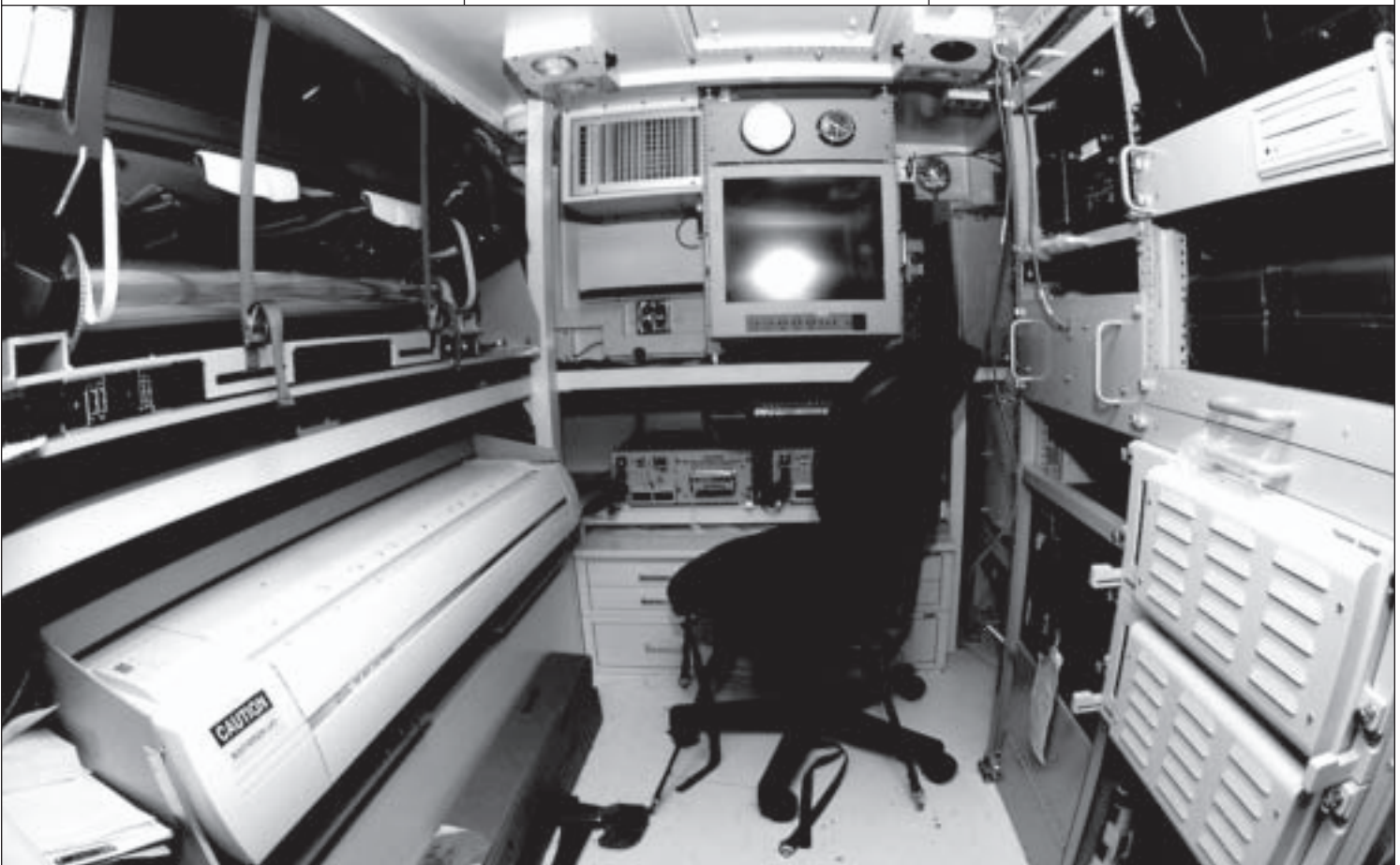
DTSS-Light, one of the four systems that make up DTSS, is a mobile terrain analysis system that is housed in a climate-controlled shelter on a Humvee. (U.S. Army photo by CTIS staff photographer.)
