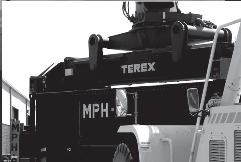
An LMM is put in place by a Rough Terrain Container Handler. (U.S. Army photo by Randy Talbot, TACOM Historian.)
