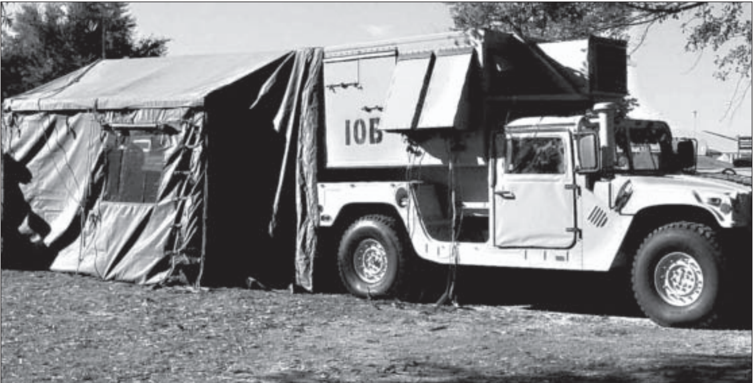
JNN is a PEO C3T nondevelopmental item rapid-acquisition effort using GOTS and COTS equipment to provide critical BLOS connectivity. (U.S. Army photo by Michael Castellana, Project Manager Tactical Radio Communications Systems.)
